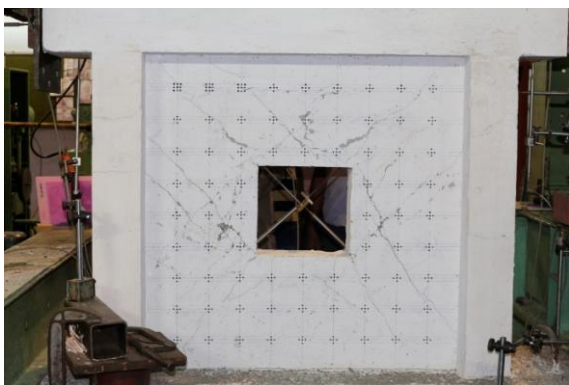
Figure 12: Crack pattern at Peak Load in SW-1.0-CW-IS
