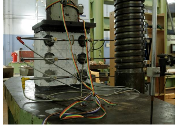
Figure 9: Experimental test set-up for strut S1-4
