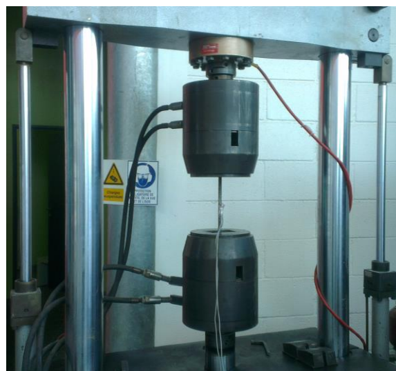
Figure2: Tensile test of reinforced steel
