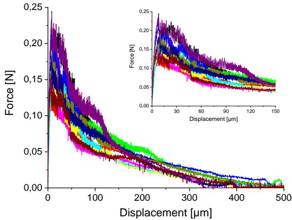
**Figure 13:** Quasi-static SFPO - AR-PU2-NC
