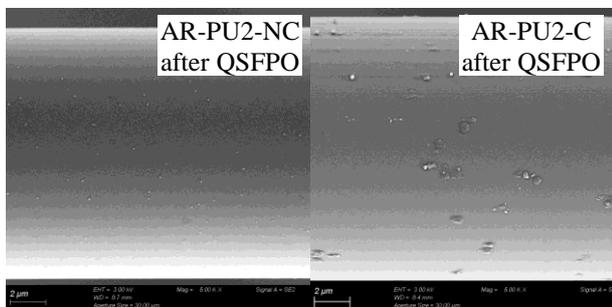
**Figure 15:** SEM images of AR-PU2-NC (left) and AR-PU2-C (right) after QSFPO
