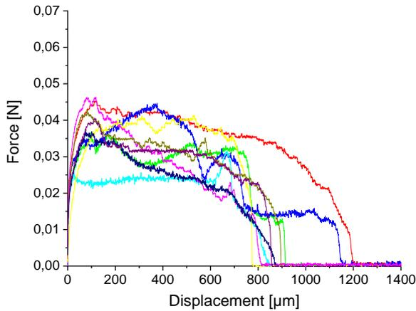
Figure 5: Quasi-static SFPO - PP-C1 (circular shape)
