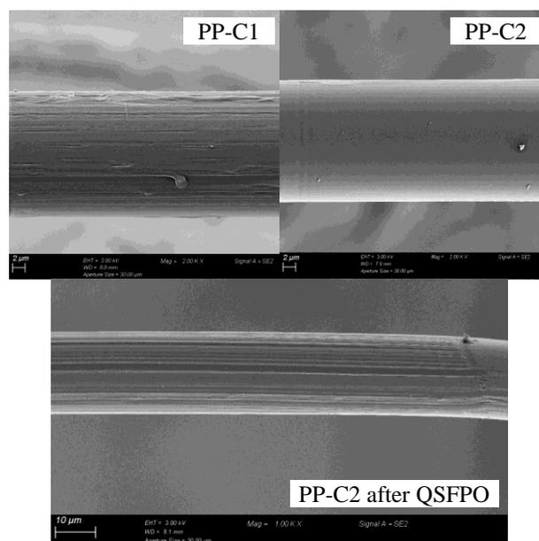
**Figure 1:** SEM images of the PP fibers, PP-C1/C2: comparison of the Surface structure in the initial state (before pull-out); PP-C2 after QSFPO: scratches due to mechanical abrasion during pull-out
