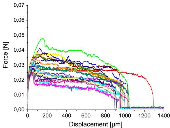
Figure 6: Quasi-static SFPO - PP-C2 (circular shape)
