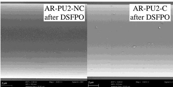
Figure 10: SEM images of AR-PU2-NC (left) and AR-PU2-C (right) surface after DSFPO
