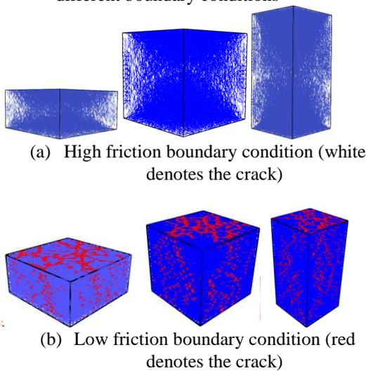
**Figure 8** Failure behavior of concrete in compression with different boundary conditions
