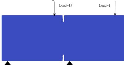
**Figure 15** Geometry of DEN beam shear test
