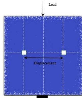
**Figure 12** Geometry of splitting test specimen
