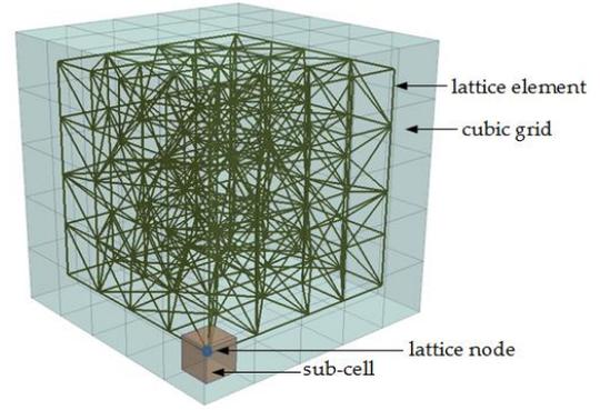
**Figure 1:** Node and mesh generation procedure of 3D lattice model
