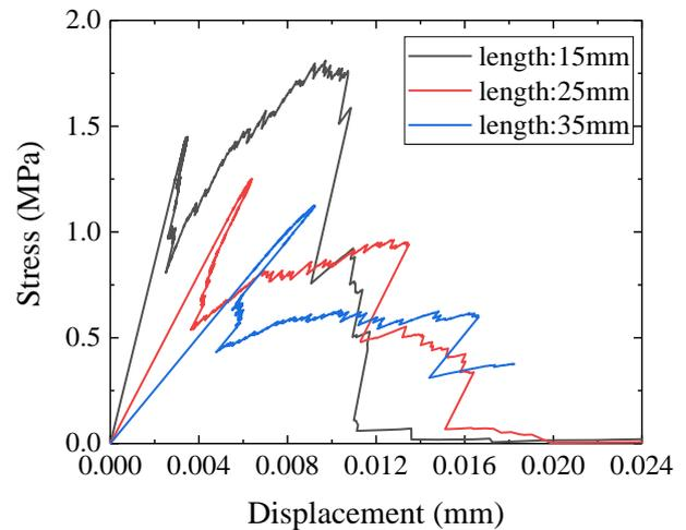
**Figure 13** Stress and displacement curve for splitting test
