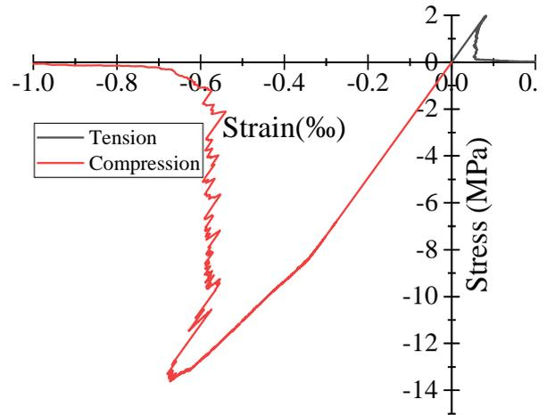
**Figure 6** The stress and strain curve of concrete exposed to uniaxial loading
