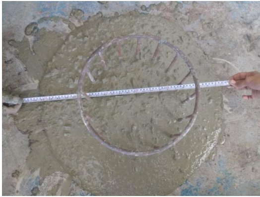
Figure 4 J - Ring Test for SCC as per EFNARC Standard
