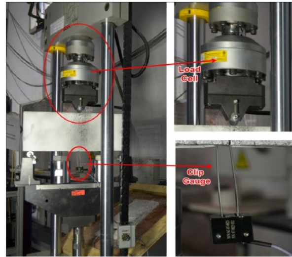
Figure 3 Closed loop Servo Controlled Test Setup used in the study
