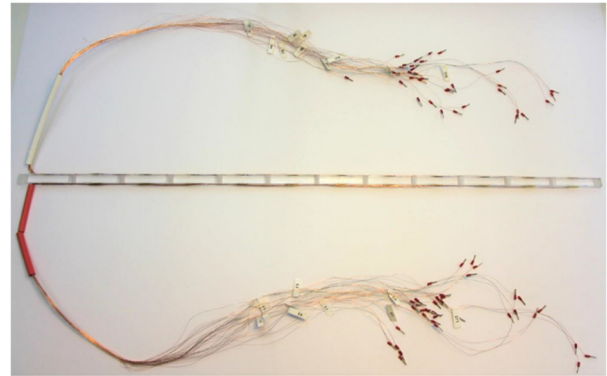
Figure 7: Acrylic rod with 24 strain gauges for the H/D = 6 specimen (Photo: N. Heider).
