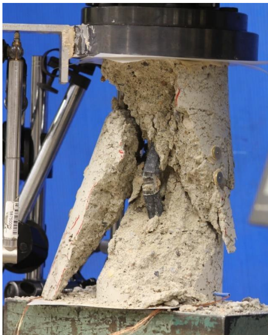
Figure 6: Acrylic rod buckling within a H/D = 2 specimen (Photo: N. Heider).
