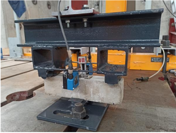
Figure 2: Flexural fatigue test.
