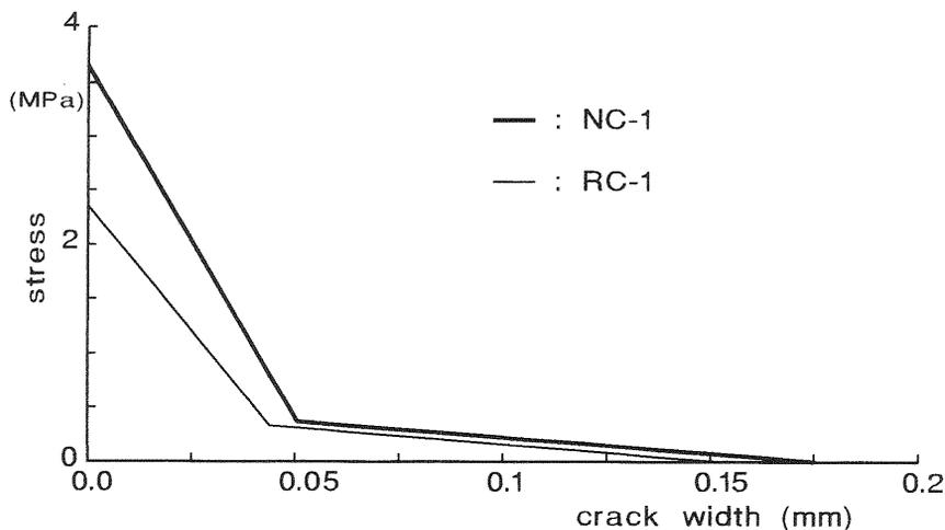
Fig. 5 Bilinear softening curves of concrete with natural (NC) and aggregate from recycled concrete (RC)
