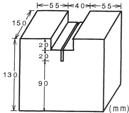
Fig.2 Size and shape of specimen
