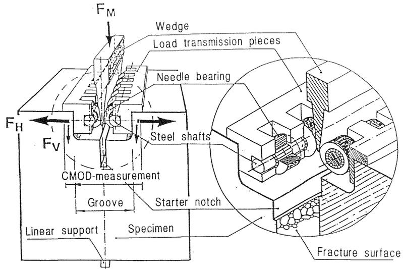
Fig.1 Principle of the testing method according to Tschegg (Tschegg 1986)
