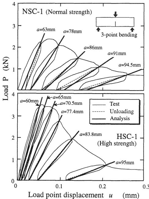
Fig. 8. Off-set test results
