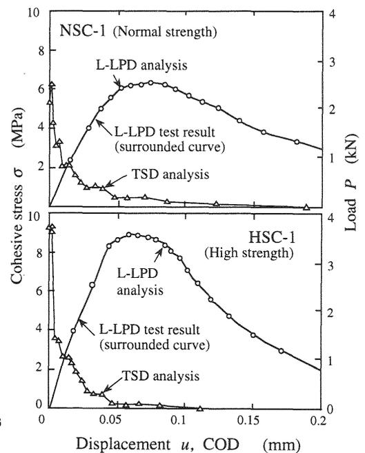
Fig. 9. L-LPD curve and TSD
