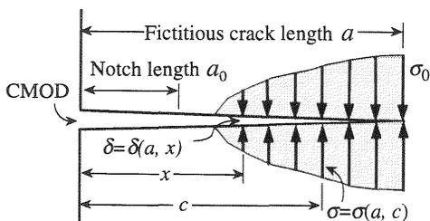
Fig. 1. Cohesive force model(CFM)
