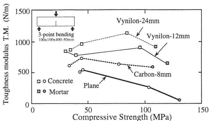
Fig. 13. Toughness modulus(T.M.) and compressive Strength
