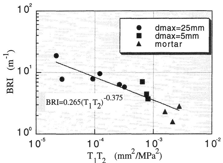
Fig. 8. Relation between brittleness parameters
