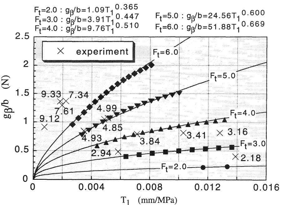
Fig. 6.  $g_\beta/b-T_1$  relationship for three point bending test
