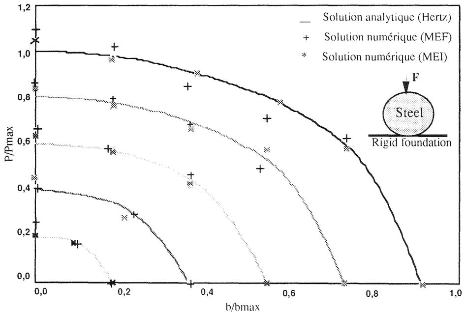
Figure 4 Comparative curves for the normal stress to the contact area:
