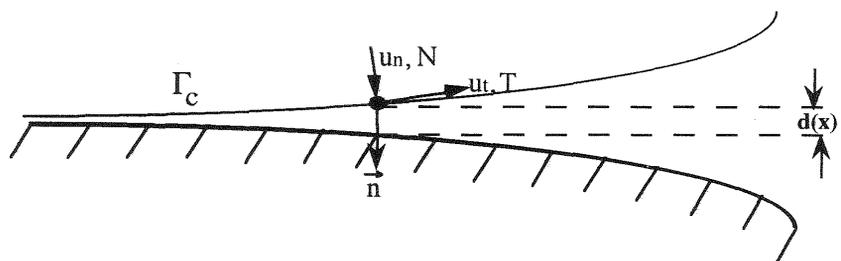
Figure 1 Contact between elastic body and rigid foundation.
