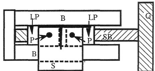
Fig. 2 Schematic of the loading stage: S --- Specimen, P--- Loading Pins, B---Base of loading stage
