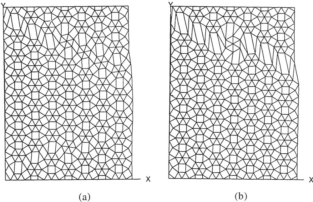
Fig. 7 (a) Deformed mesh at 77% of the prescribed maximum strain; (b) deformed mesh at 100% of the prescribed maximum strain
