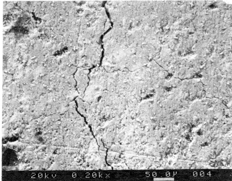
Fig. 4 Crack branch and crack bridging in the wake of crack
