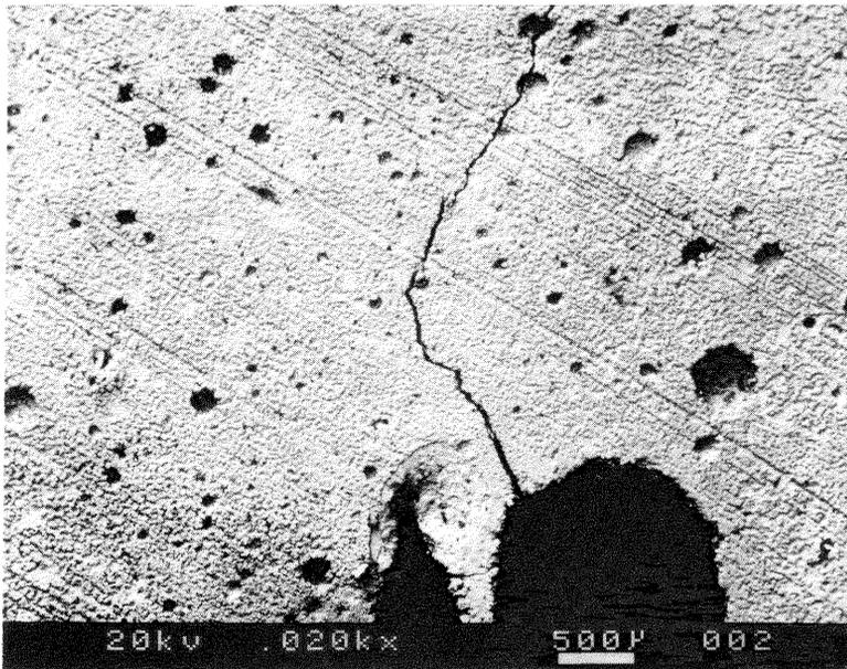
Fig. 3 Crack propagation from the crack tip
