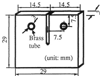
Fig. 1 Geometry of compact-tension specimen
