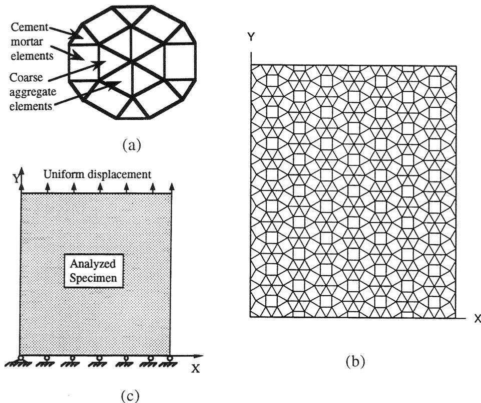
Fig. 5 (a) Coarse aggregate and mortar elements; (a) Finite element mesh for complete specimen; (c) Boundary conditions for the computational specimen
