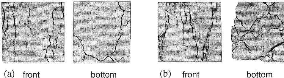
Fig. 5. Crack patterns for 100 mm NSC specimen loaded under HF (a) and LF boundary conditions (b)
