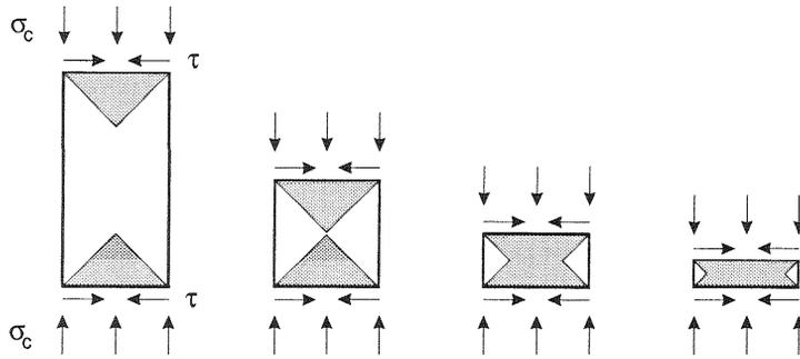
Fig. 4. Confined zones for different specimen heights due to boundary friction
