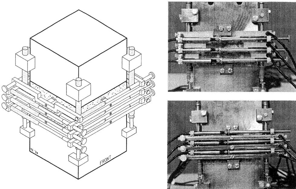
Fig. 2. Experimental set-up for compression tests,  $L_{\text{specimen}}=50$  mm
