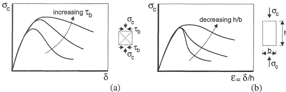
Fig. 1. Effect of specimen slenderness (a) and boundary restraint (b) on the compressive stress-deformation behaviour of concrete (Van Vliet and Van Mier, 1994)
