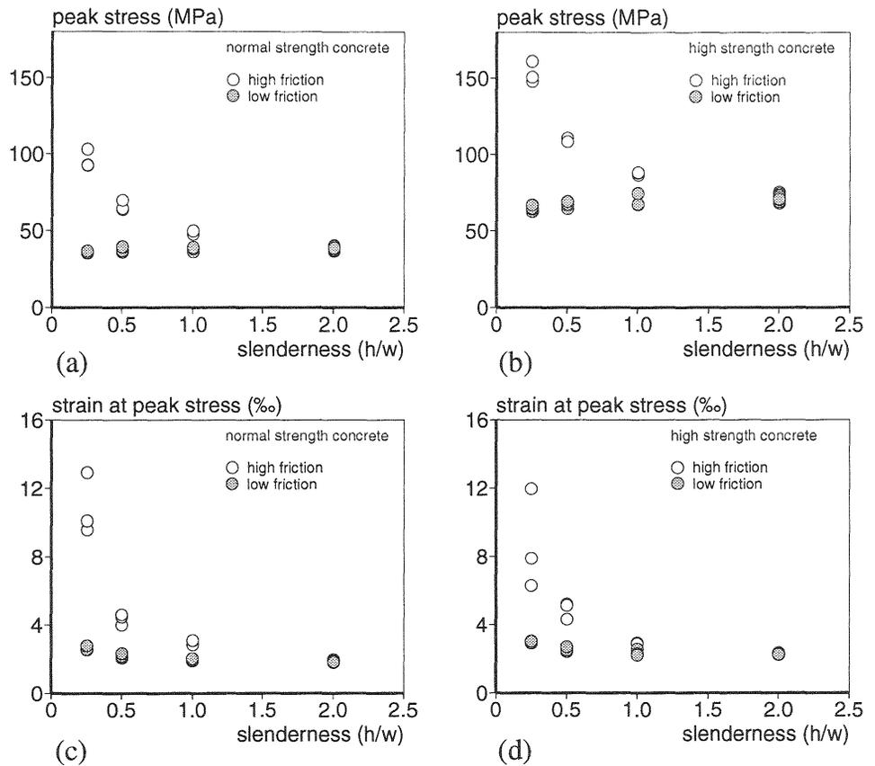
Fig. 7. Peak stresses (a,b) and strains (c,d) for NSC (a,c) and HSC (b,d)
