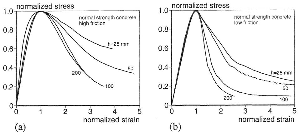
Fig. 9. Normalized stress-strain curves for the normal strength concrete
