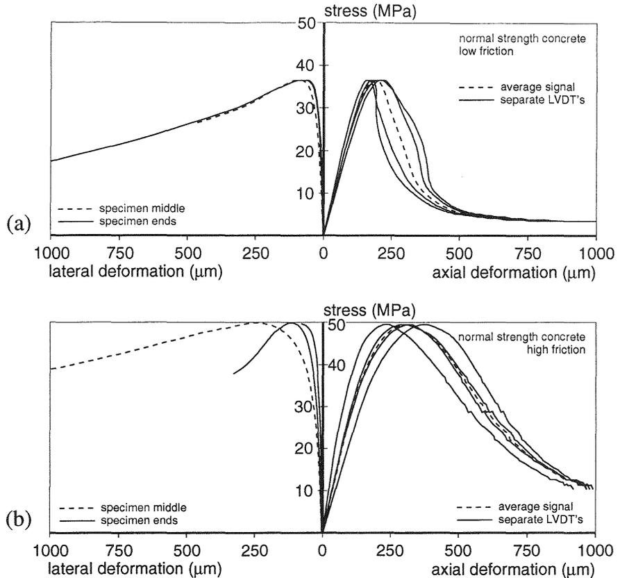
Fig. 6. Axial and lateral deformations of 100 mm NSC specimen under LF (a) and HF boundary conditions (b)
