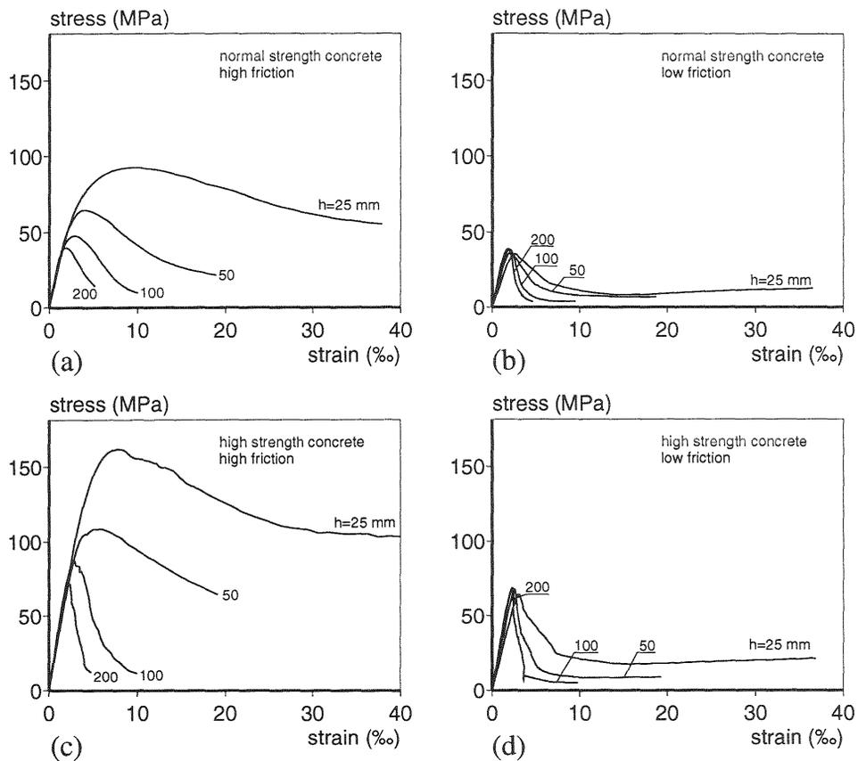
Fig. 3. Stress vs. axial strain for the NSC (a,b) and HSC (c,d) tested under HF (a,c) and LF boundary conditions (b,d)
