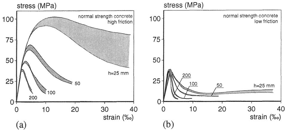
Fig. 8. Range of results NSC specimens with HF and LF boundaries
