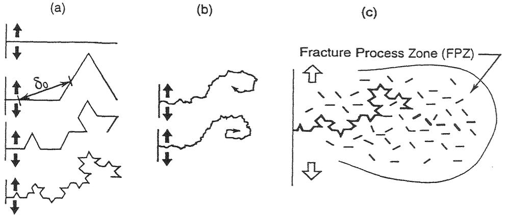
Figure 1: Von Koch curves as examples of fractal crack at progressive refinement; (b) recessive and spiraling segments which can be exhibited by fractal path; (c) fractal crack forming in a fracture process zone.
