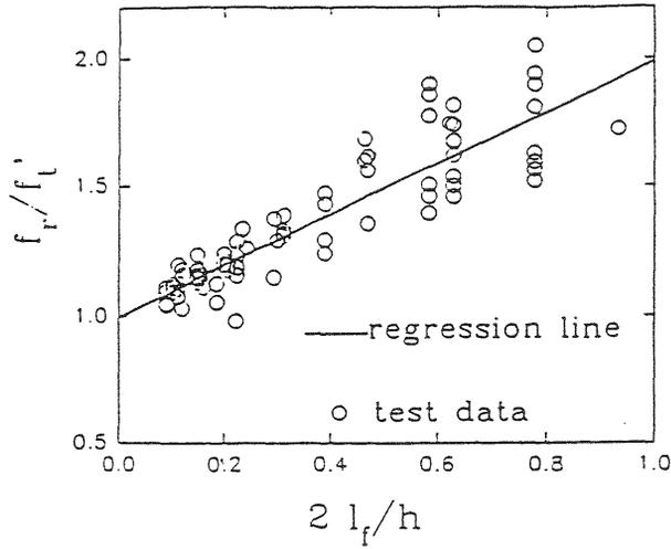
Figure 5: Test data for the dependence of modulus of rupture  $f_r$  of unreinforced concrete beams on beam depth  $D$ , and their optimum fit by the nonfractal formula (6);  $f_t'$  = direct tensile strength,  $h = D =$  beam depth,  $l_f =$  constant (after Bažant and Li, 1993).
