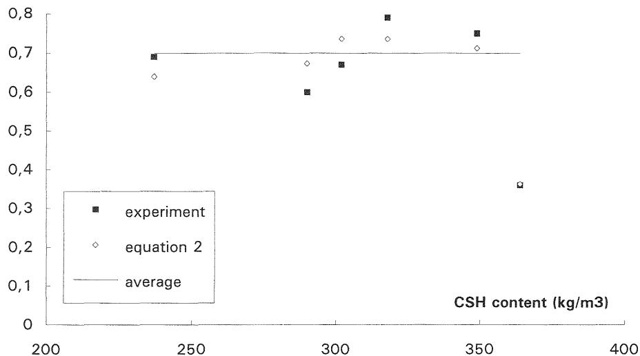
Fig. 5. Experimental values of  $\alpha$  and prediction using eq. 2.
