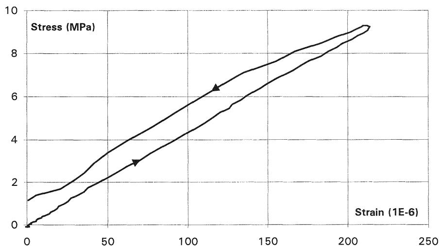
Fig. 1. Stress-strain evolution for mini-concrete tested at 60 GPa/s
