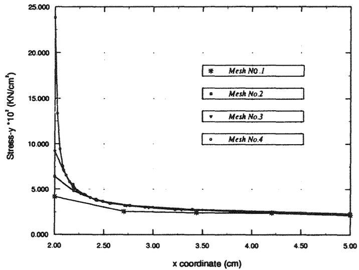
Fig. 7. Stress  $\sigma_y$  curves along cracked line(x axis) for different meshes
