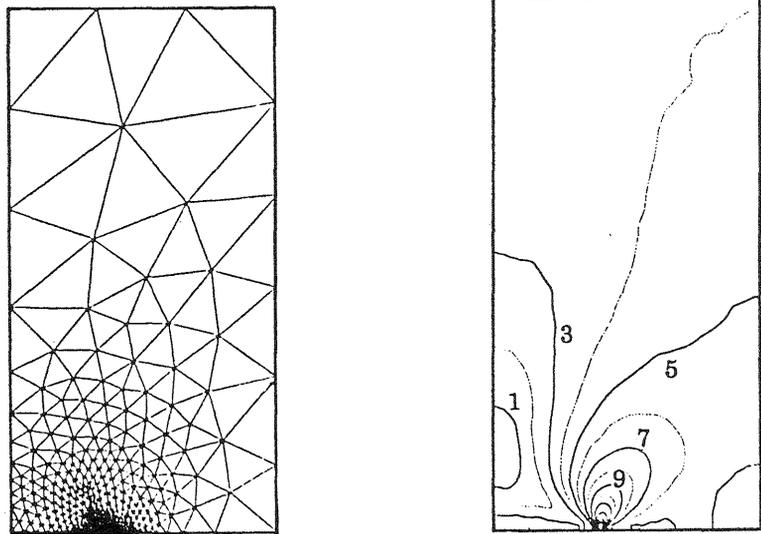
( a ) refined mesh(N=398, E=722) ( b ) stress contours( $\eta_{spe} \approx 1\%$ )
