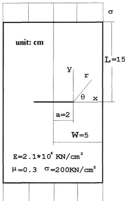
Fig. 2. a centre cracked panel
