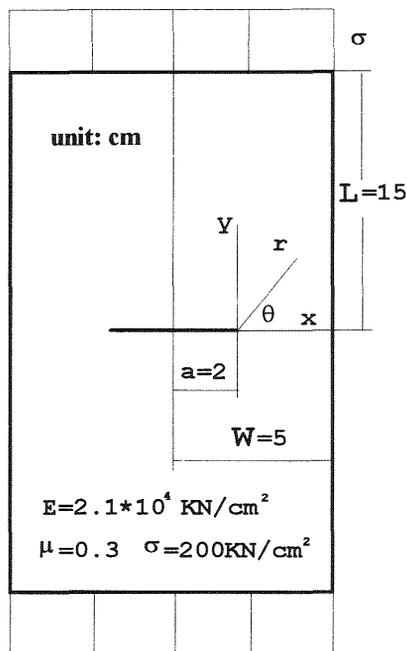
Fig. 2. a centre cracked panel
