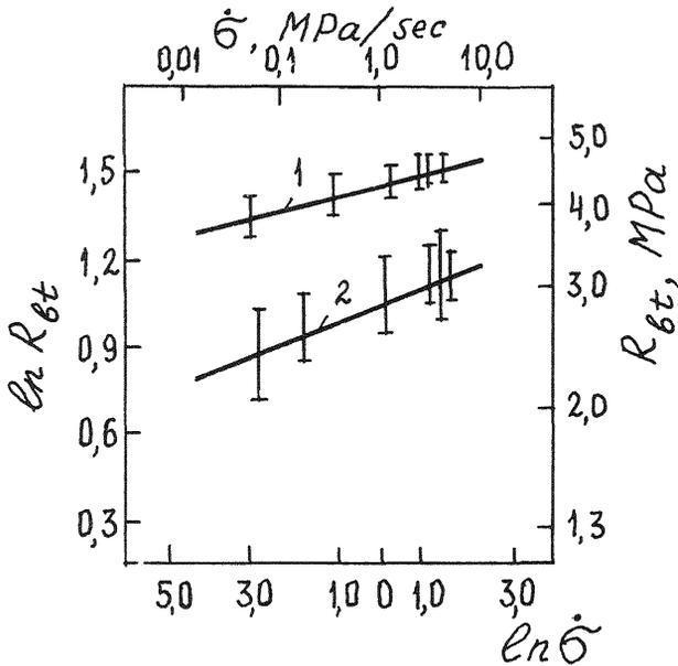
Fig. 1. Concrete tensile strength at bending as a function of stressing (loading) rate  $\dot{\sigma}$ ; 1 - before heating and 2 - after heating up to 800°C.
