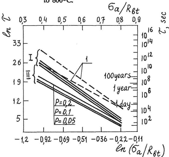
Fig. 2. Time to failure of concrete ( $\bar{\tau}$ ) depending on heating temperatures and stress applied; I - before heating; II - after heating at 800°C; 1 -  $\bar{\tau}$ , calculated according to equation (1).
