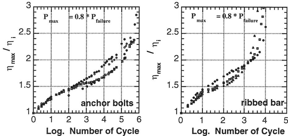
Fig. 6. Displacement referred at first cycle as a function of number of cycles of two types of anchor
