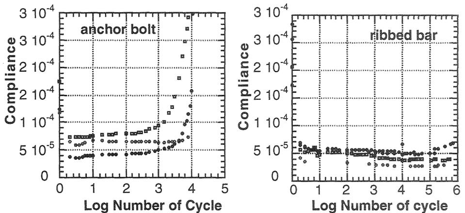
Fig. 5. Compliance vs. number of cycles of two types of anchor
