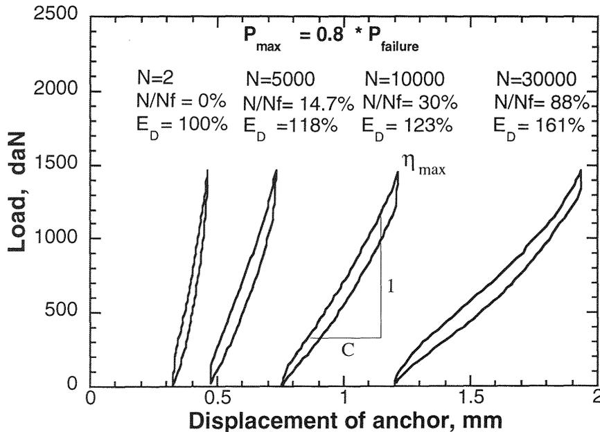
Fig. 3. Variation of cycle shape in fatigue test.
