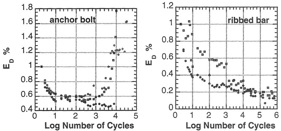
Fig. 4. Energy dissipated per cycles referred at  $2^\circ$  cycle vs number of cycles of two types of anchor
