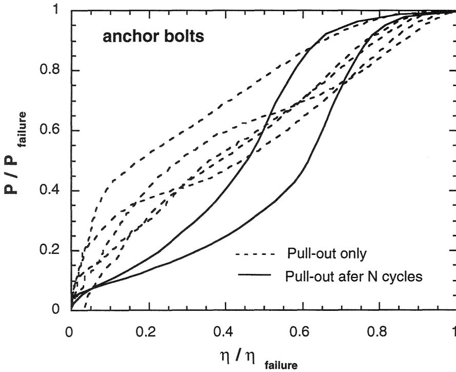
Fig. 8. Dimensionless load versus dimensionless displacement
