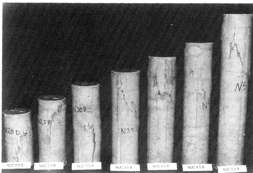
Fig. 13 - Effect of height to length ratio on the strain softening behavior for L:D from 2.0 to 5.5
