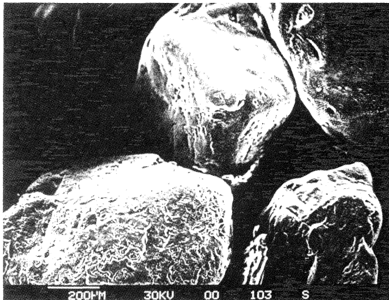
Fig. 5. SEM photographs showing the roundish shape of the sand grains.
