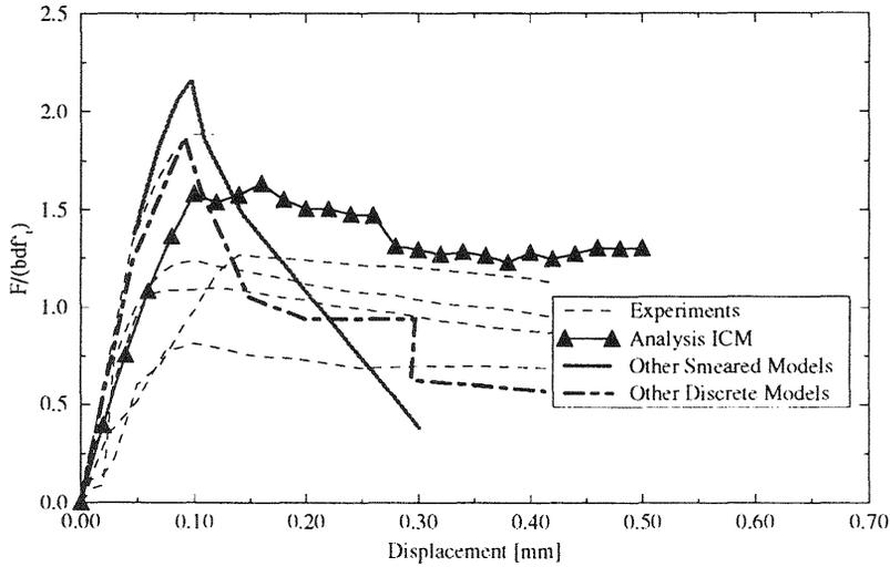
Figure 7: Load displacement curve for test I.
