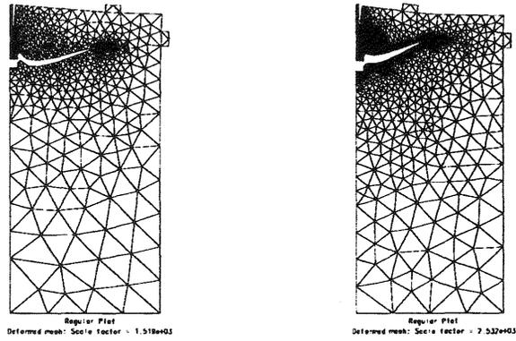
Figure 2: Final crack pattern for anchor bolt pull out tests.
