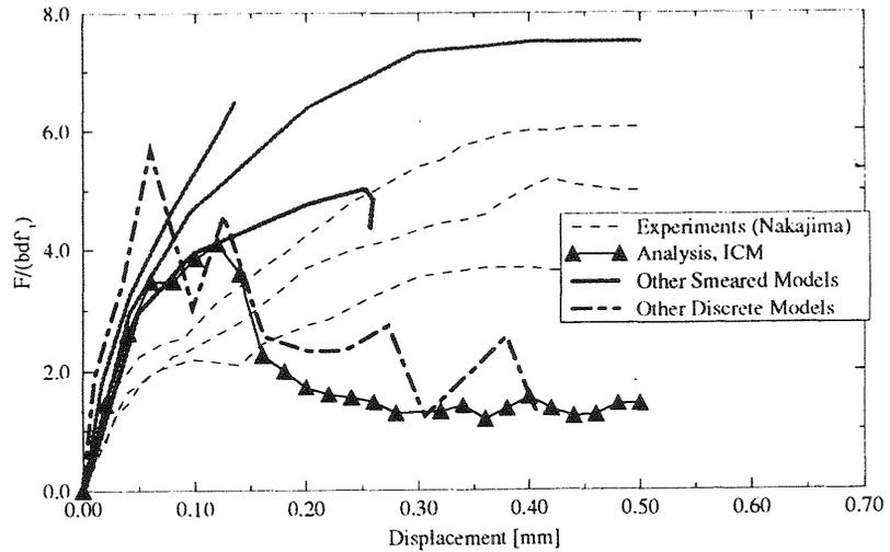
Figure 8: Load displacement curve for test II.
