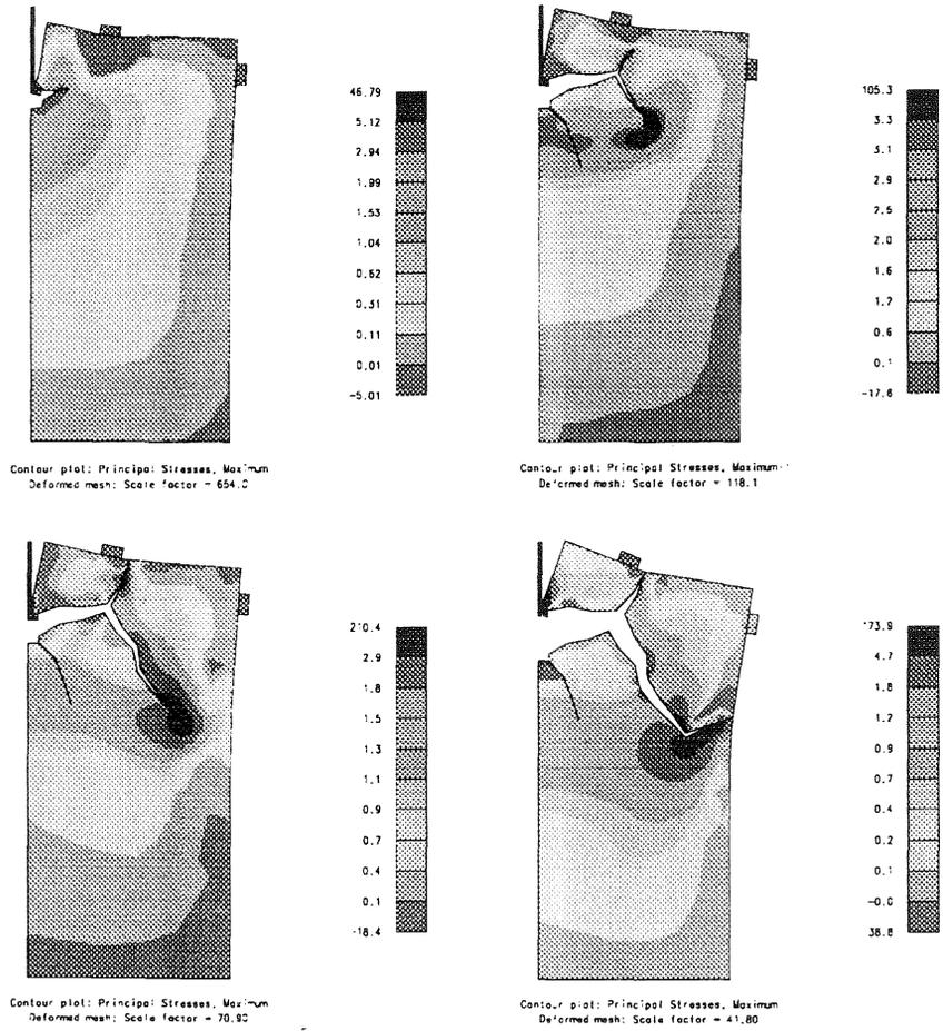
Figure 5: Crack propagation for anchor bolt pull out test II.
