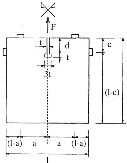
Figure 1: Anchor bolt pull out test geometry.
