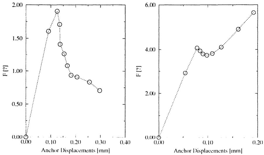
Figure 3: Load displacement curves for anchor bolt pull out tests.
