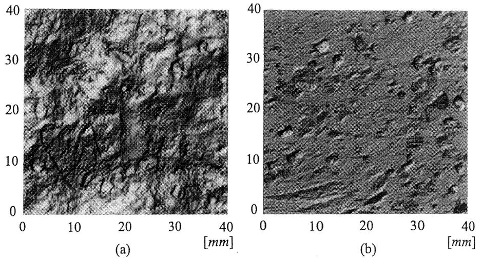
Fig. 2. Shaded reliefs: fracture surface (a), plane cross-section (b).
