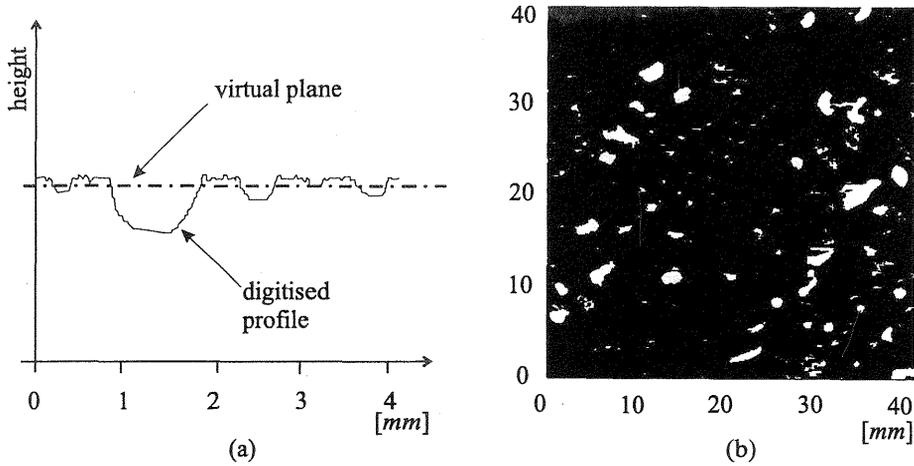
Fig. 7. Virtual plane section scheme (a) and bidimensional map of the effective cross section (b).
