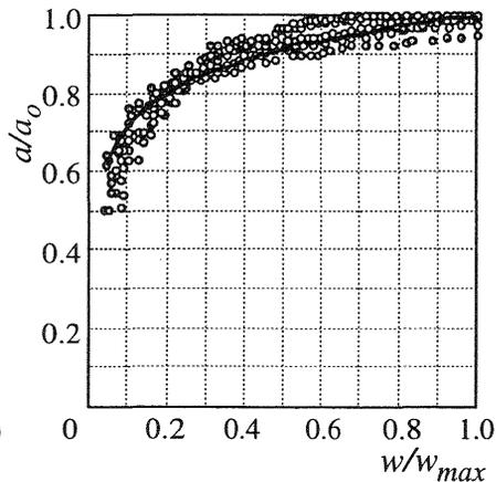
Fig. 10. Fictitious crack length and crack mouth opening relation
