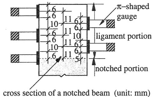
Fig. 8. Arrangement of  $\pi$ -shaped gauges
