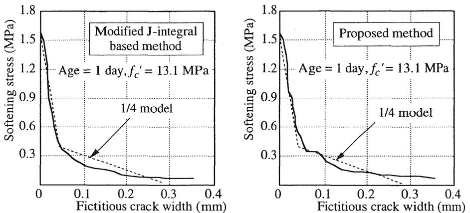
Fig. 13. Tension softening curve of normal strength concrete
