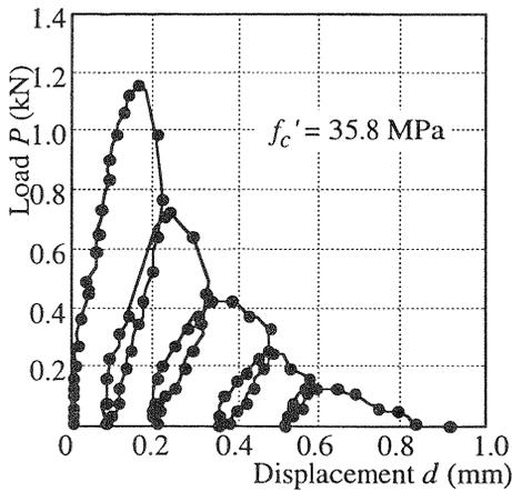
Fig. 5. Load-displacement relation (Normal strength concrete, 28 days)
