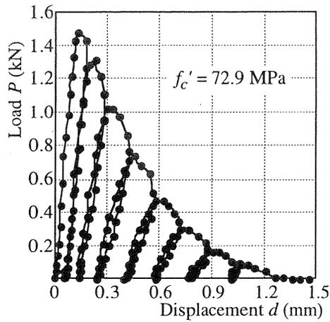
Fig. 4. Load-displacement relation (High strength concrete, 3 days)
