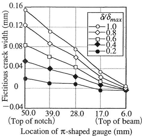
Fig. 9. Distribution of fictitious crack width (Self-compacting concrete, 28 days)
