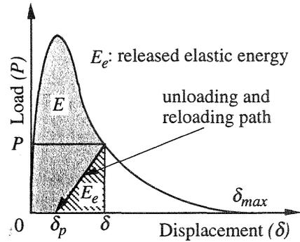
Fig. 2. Release of elastic energy
