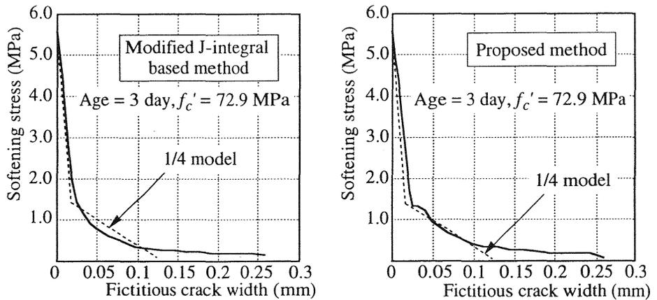
Fig. 12. Tension softening curve of high strength concrete
