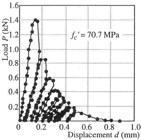
Fig. 3. Load-displacement relation (Self-compacting concrete, 28 days)
