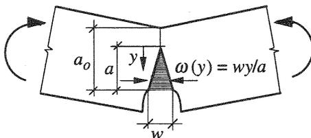
Fig. 7. Propagation of a fictitious crack
