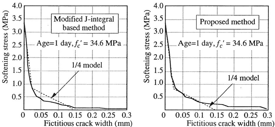
Fig. 11. Tension softening curve of self-compacting concrete
