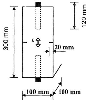
Fig. 1. Geometry of specimen.
