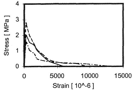
Fig. 2. Typical stress-strain curves of concrete in tension.
