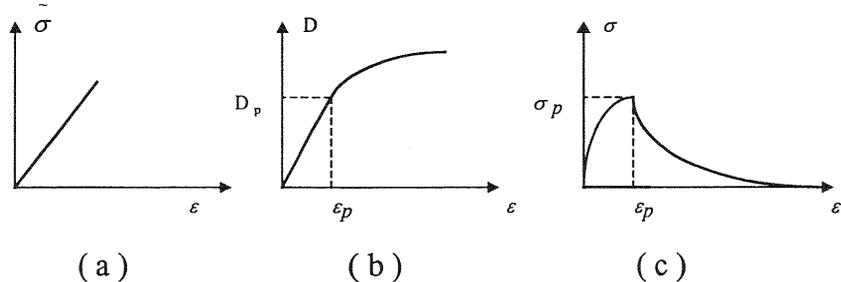
Fig. 4. Schematic illustrations of  $\tilde{\sigma}$  vs.  $\varepsilon$ ,  $D$  vs.  $\varepsilon$ , and  $\sigma$  vs.  $\varepsilon$ .
