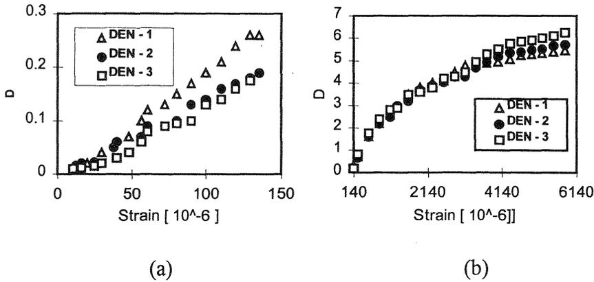
Fig. 3. Damage  $D$  vs. concrete strain  $\varepsilon$  before (a) and after (b) peak load.
