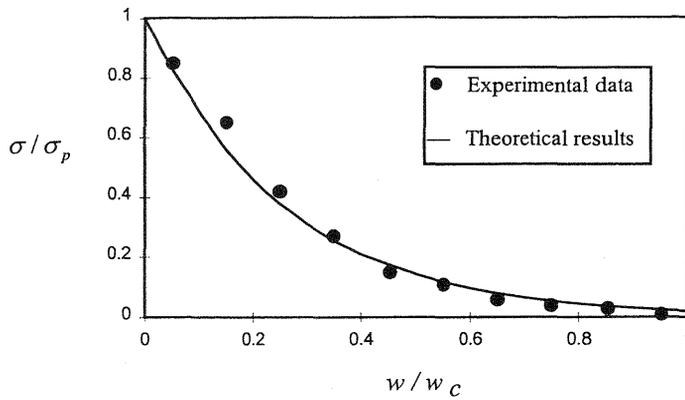
Fig. 8. Comparison between experimental data of Gopalaratnam and proposed model curves for the concrete.
