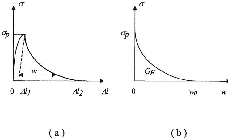
Fig. 5. Stress -deformation curve and strain softening curve.
