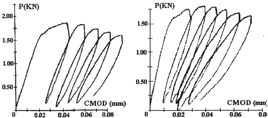
Fig. 3 Plots of P x CMOD tests (note different scales).
