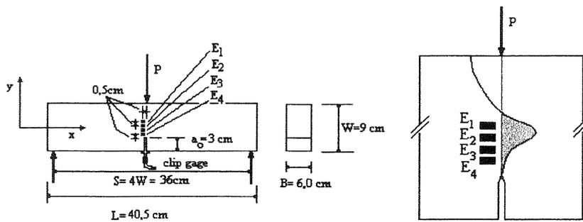
Fig. 4 Extensometric arrangement in a three point bending beam and expected stress distribution
