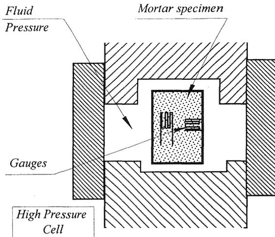
Fig. 5. Experimental hydrostatic test principles.
