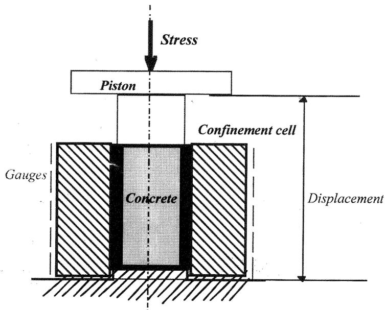
Fig. 1. Principles of the uniaxial confined compression test.
