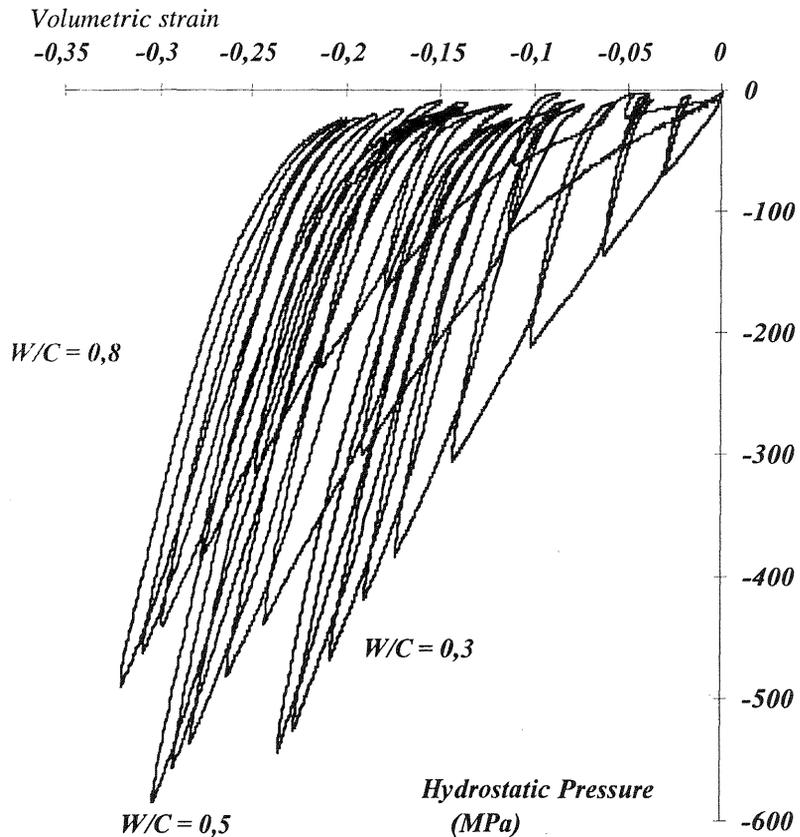
Fig. 3. Hydrostatic stress versus volumetric strain (percent) obtained on different mortars (W/C = 0.3 ,0.5, 0.8) .
