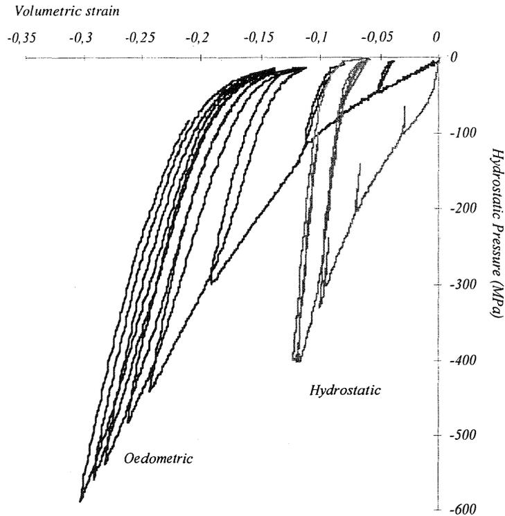
Fig. 7. Experimental hydrostatic and oedometric test results on mortar.
