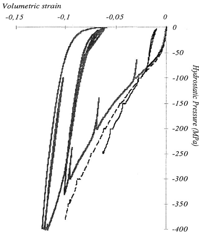
Fig. 6. Hydrostatic pressure versus volumetric strain (percent) curves for mortar.
