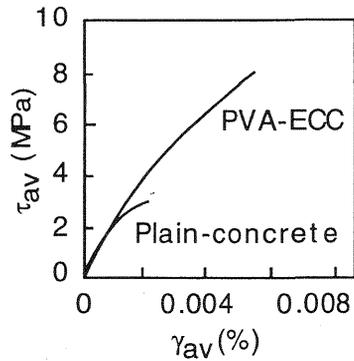
Fig. 10 Shear load capacity
