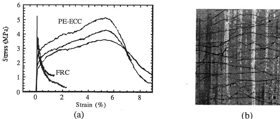
Fig. 2 (a) Uniaxial tensile behavior of ECC, and (b) microcracking with spacing of about 1mm on tension specimen.
