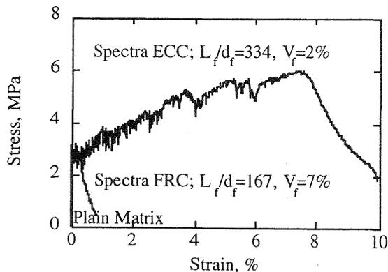
Fig. 1. Stress-strain curves demonstrating the importance of  $V_f^{crit}$
