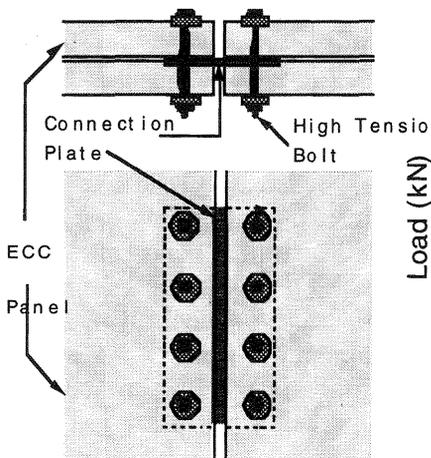
Fig. 11 Dry joint configuration
