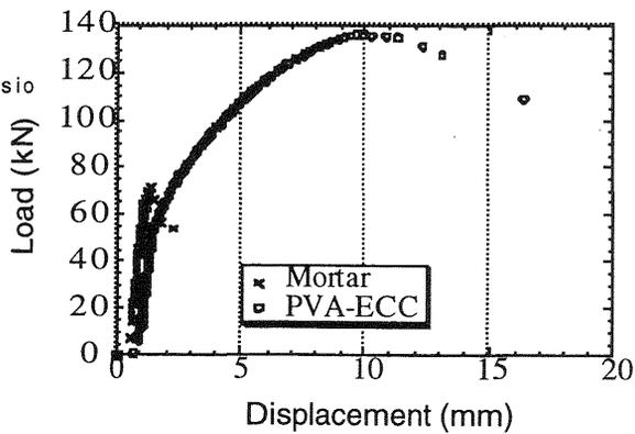
Fig. 12 Load-displacement curve of indent test
