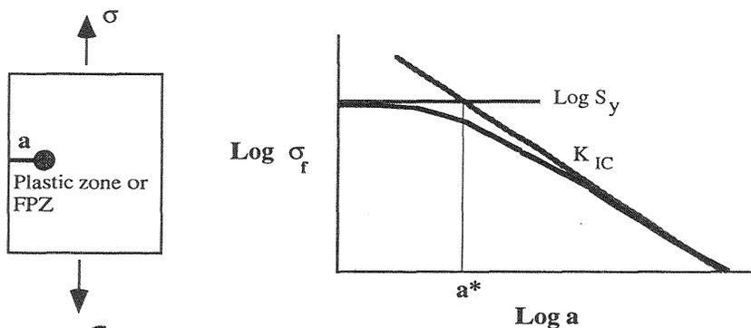
Fig. 1. Tensile failure of a large metal plate with a small edge crack
