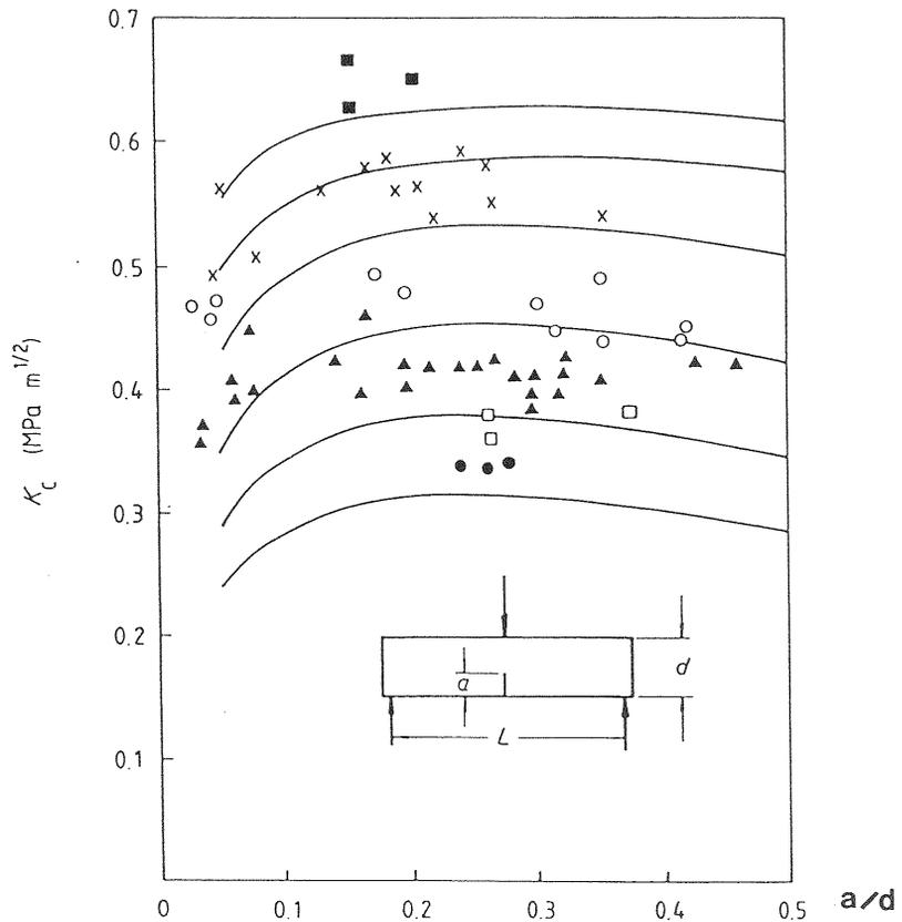
Fig. 2. Critical stress intensity factor as function of  $a/d$  ratio.  $d$  (mm) = 5 ●, 8 □, 14 ▲, 28 ○, 56 ×, 110 ■, after Cotterell and Mai (1987, 1996) and Higgins and Bailey (1976)
