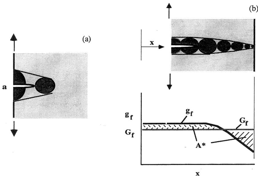
Fig. 4. (a) Contour of FPZ for short edge cracks and (b) contour of FPZ for cracks close to the free back surface.
