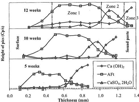
Figure 3. Identification by XRD analysis of the solid compounds in the degraded zone of the cement paste samples at different times
