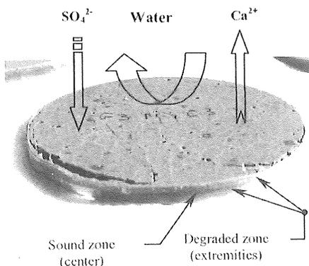
Figure 1. Sulfate attack with calcium leaching of a CPA-CEM I cement paste sample
