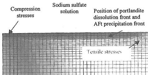
Figure 12. Auto-stresses generated by the internal precipitation of AFt in the calcium depleted part of the sample
