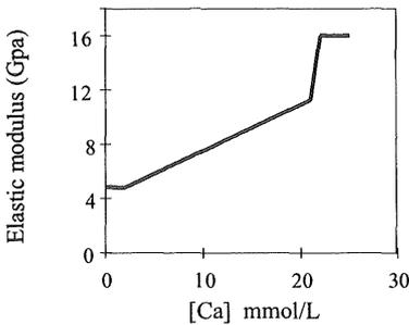
Figure 8. Evolution of the elastic modulus with the calcium ionic concentration.
