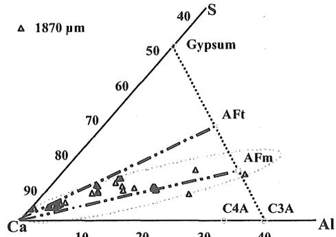
Figure 4. Cement paste composition before testing, obtained from EDS micro-analysis
