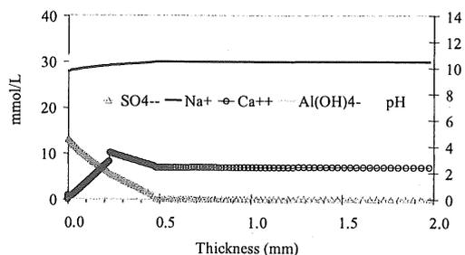
Figure 7. Simulated profiles of concentrations in liquid phases after 3 weeks of testing.
