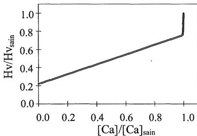
Figure 9. Evolution of the normalized cohesion with the normalized calcium ionic concentration.
