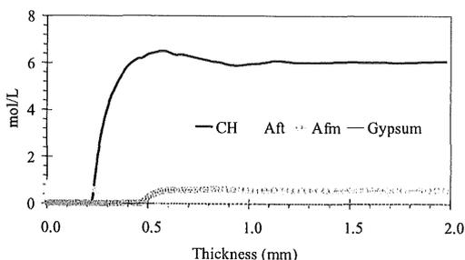
Figure 6. Simulated profiles of concentrations in solid phases after 3 weeks of testing.
