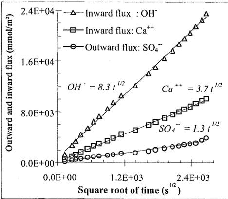
Figure 2. Inward and outward fluxes of calcium, hydroxyl and sulfate ions
