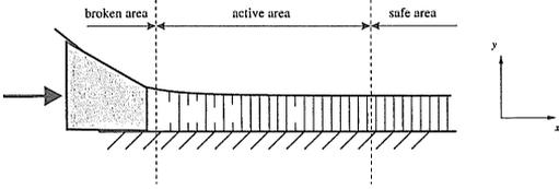
Figure 1: A schematic representation of the ‘‘Zip’’ model. The point where the displacement is imposed may move along the  $x$ -axis.
