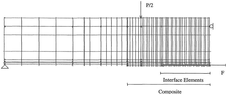
Figure 4. The Finite Element Mesh used in our Analysis
