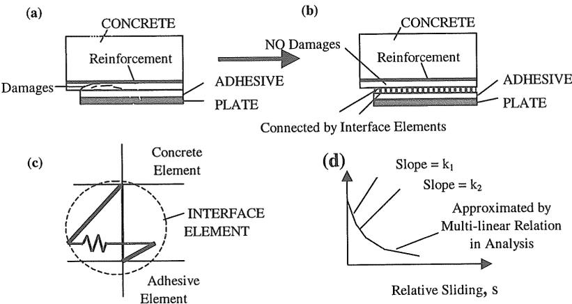
Figure 1 (a) and (b) Representation of concrete damage with non-linear interface elements (c) the interface element, (d) Variation of element shear stress with sliding
