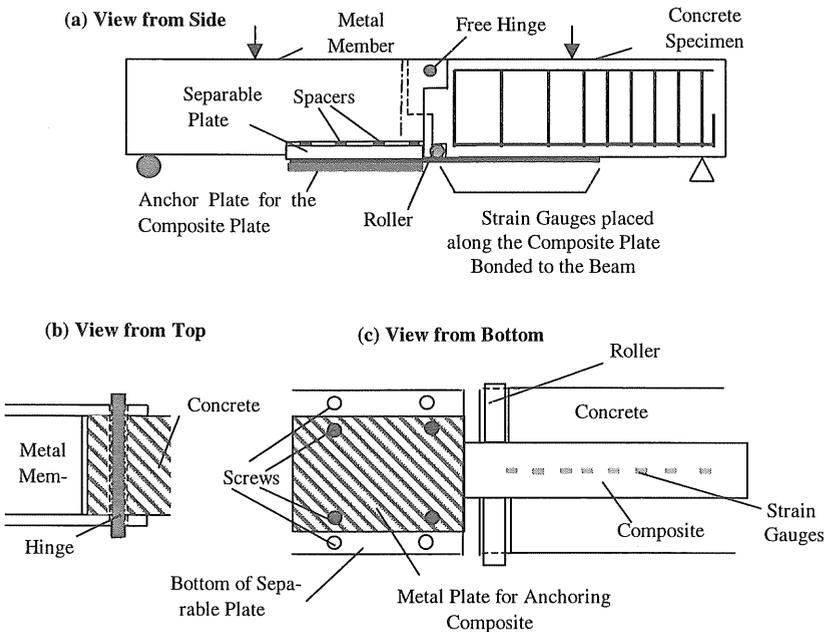
Figure 2. Experimental Set-up to Determine Constitutive Relation of the Interface Element
