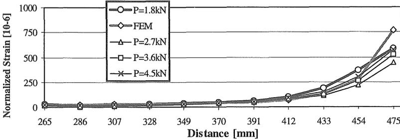
Figure 5. Comparison between Normalized Experimental and FEM results for P up to 4.5 kN
