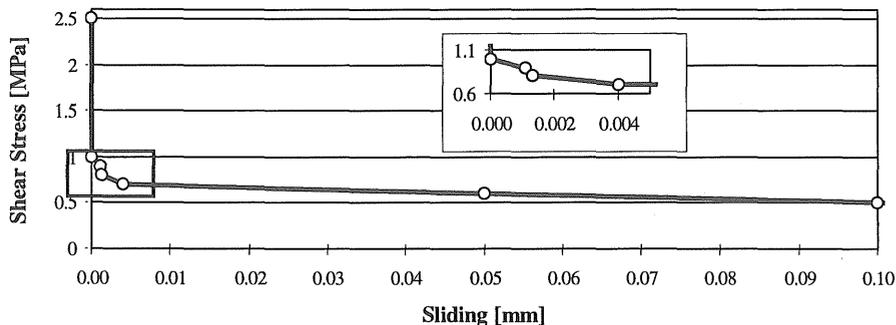
Figure 8. The Experimental Determined Interfacial Softening Relation
