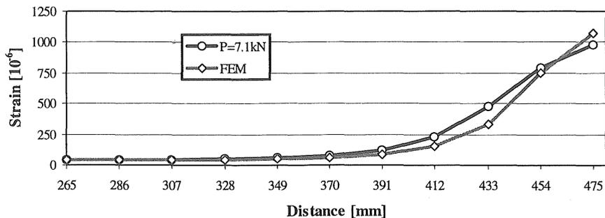
Figure 6. Comparison between Experimental and FEM results for P = 7.1 kN
