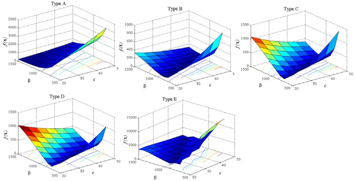
Figure 3. Objective function  $f(\mathbf{x})$  for different specimen sizes. In all cases  $\alpha = 0.93$ .
