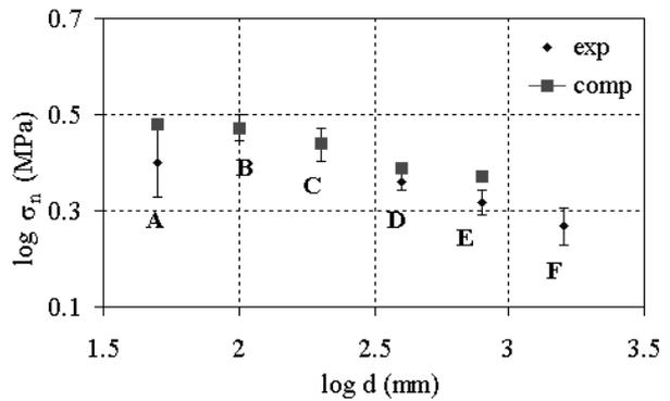
Figure 8. Experimental and computational nominal strength  $\sigma_n$  vs. specimen size  $d$ .
