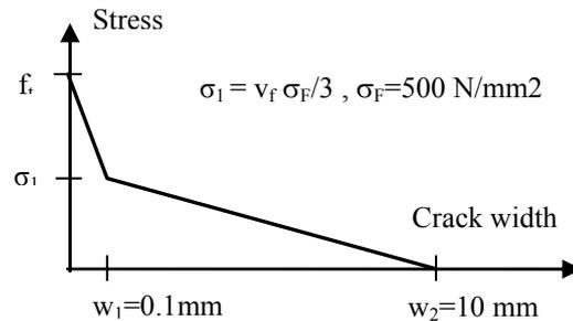
Figure 3. Stress-crackwidth relation used in the present study
