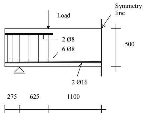
Figure 1. Geometry of the largest beam
