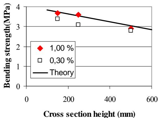
Figure 8. Bending strength vs cross section height
