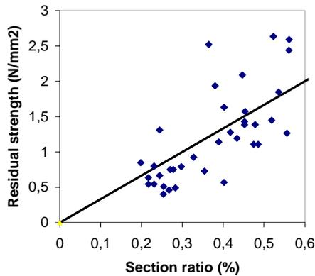
Figure 7. Residual strength versus measured section ratio for small beams (Series IV,  $b/h=150/150$ ).
