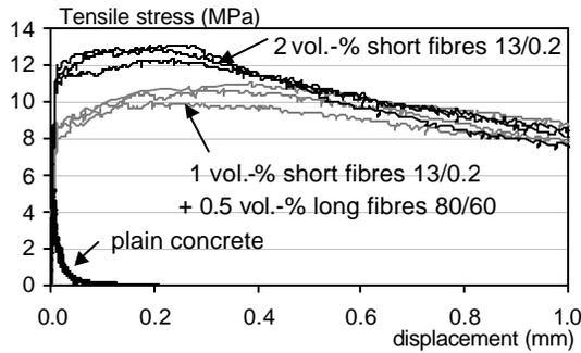
Fig. 6: Comparison of tensile response of concrete with only short fibres and with somewhat lower amount of short and long fibres
