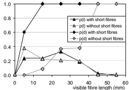
Fig. 12: Probabilities  $p(l)$  that a fibre with visible length  $l$  may be found in cracked cross-section and  $p(d)$  that fibre hooks will be deformed, for concretes with long fibres only and with long and short fibres
