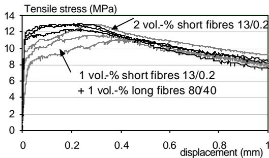
Fig. 7: Comparison of tensile responses of concrete with only short fibres, and concrete with the same amount of short and long fibres
