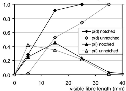
Fig. 13: Probabilities  $p(l)$  that a fibre with visible length  $l$  may be found in cracked cross-section and  $p(d)$  that fibre hooks will be deformed, for notched and un-notched specimens of the same type of Hybrid-Fibre Concrete
