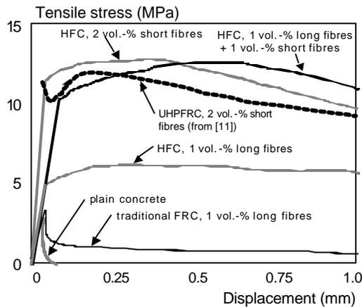
Fig. 10: A schematic comparison of tensile response for different types of traditional and high-performance fibre concrete
