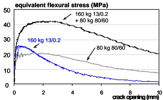
Fig. 1: Influence of short (13/0.2) and long (80/60) fibre types on flexural behaviour (from [2])
