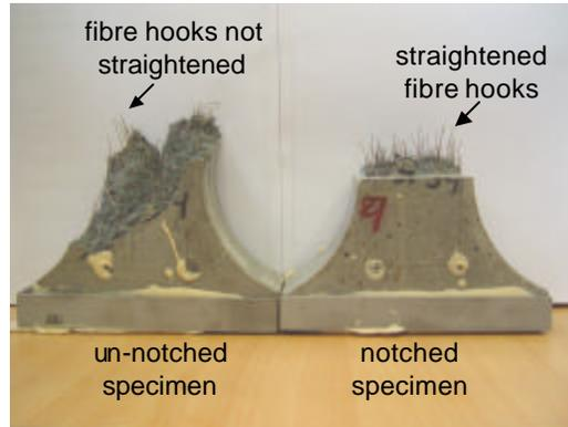
Fig. 8: Cracking patterns, position of fibres and deformation of fibre hooks in the cracking plane for un-notched and notched specimen.
