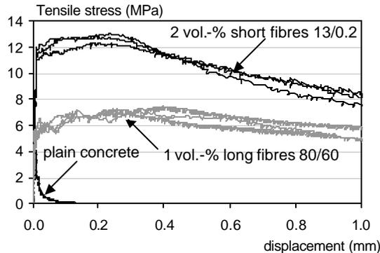
Fig. 5: Tensile behaviour of plain concrete and concrete's with a single fibre type (short or long fibres)
