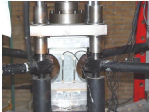
Fig. 3: Specimen with LVDT's glued in the testing frame, both ends were additionally stiffened by steel stripes outside and inside the specimen.
