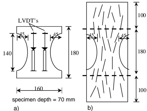
Fig. 2: a) Dimensions of the specimens with LVDTs positions, b) initial shape of the specimens with schematized fibre dispersion
