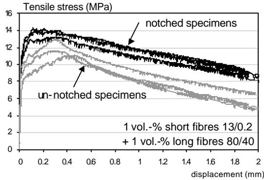
Fig. 9: Comparison of tensile response of notched and un-notched specimens of concrete No. 5 (contains both short and long fibres)
