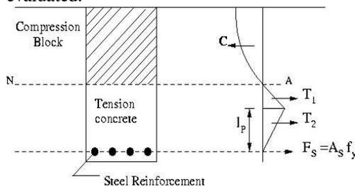
Figure 7: Stress-strain variation in a reinforced concrete section (compression and tension)
