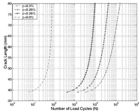
Figure 4: Crack propagation curve for reinforced concrete specimen for different reinforcement ratios
