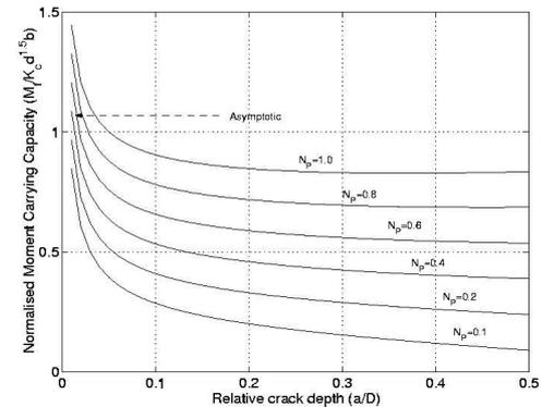
Figure 6: Moment carrying capacity with different  $N_p$  values
