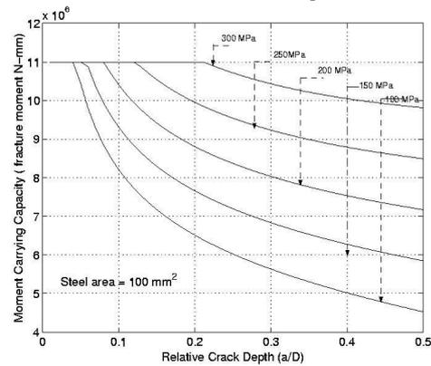
Figure 9: Design moment curves for varying stress in steel rebars (constitutive law for concrete in compression is parabolic-linear)
