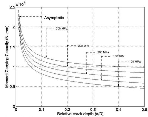
Figure 5: Moment carrying capacity for different steel force
