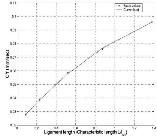
Figure 1: Relation between  $Cf$  and the ratio of ligament length to characteristic length
