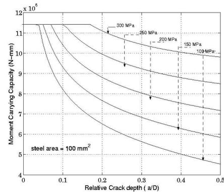
Figure 8: Design moment curves for varying stress in steel rebars (constitutive law for concrete in compression is bi-linear)
