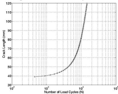
Figure 3: Crack propagation curve for reinforced concrete specimen
