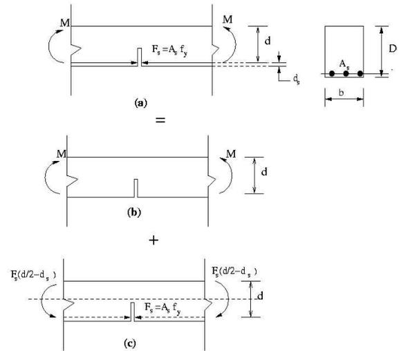
D= Overall Depth; d = Effective Depth; b = Width;  $d_s$  = Effective Cover; M = Bending Moment;  $F_s$  = Steel Force;  $A_s$  = Steel Area; Figure 2: Cracked beam element model for reinforced concrete
