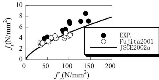
Fig.2 Compressive strength-Tension strength relation
