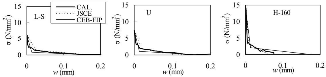
Fig.6 Tension softening curve
