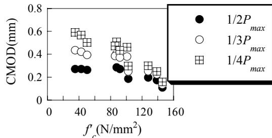
Fig.5 Compressive strength-CMOD relation
