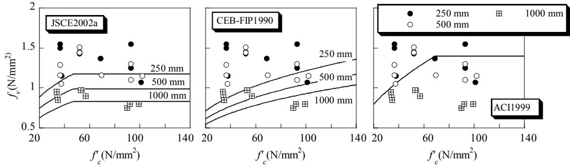
Fig.9 Compression of design code formulas with test results
