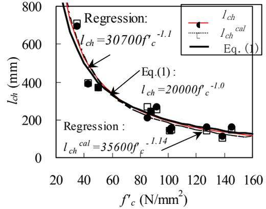
Fig.8 Dependence of compressive strength on characteristics
