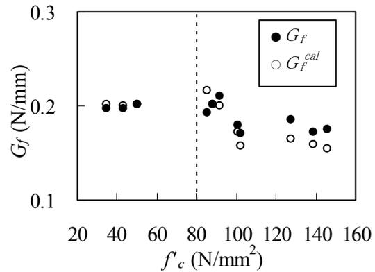
Fig.7 Compressive strength-Fracture energy relation
