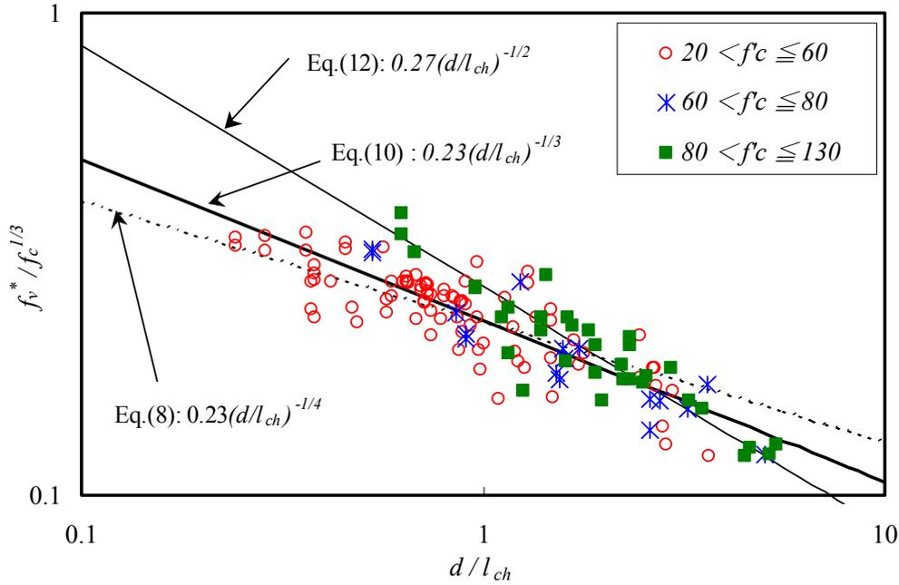
Fig.10 Study of size effect fracture mechanics with existing tests data
