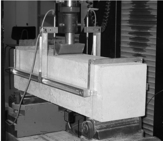
Figure 2. Experimental setup for the TPBT.
