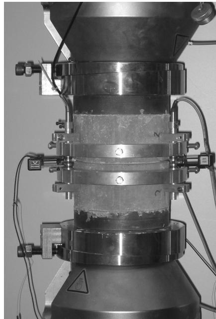
Figure 1. Experimental setup for the UTT.
