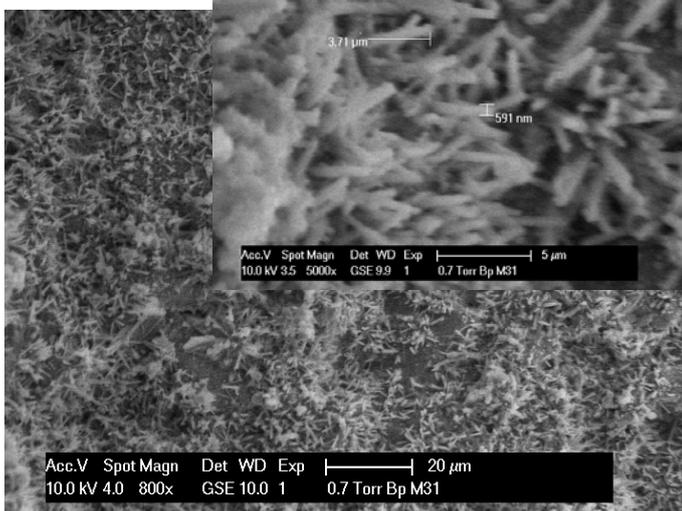
Figure 2. Concrete samples incubated in yeast extract- and peptone-containing medium. A: Control (concrete with no bacteria added) and B: Concrete containing  $10^9 \text{ cm}^{-3}$  *B.pseudofirmus* endospores. The inset in Figure 2B (5000x magnification) shows a close up of the massive calcite-like crystals formed on the concrete surface.
