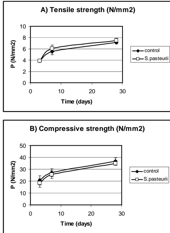
Figure 1. Flexural tensile- (A) and compressive- (B) strength testing, after 3, 7 and 28 days curing, revealed no significant difference between control- and bacterial concrete. The latter contained  $1.14 \cdot 10^9$  *S.pasteurii* cells  $\text{cm}^{-3}$  concrete.
