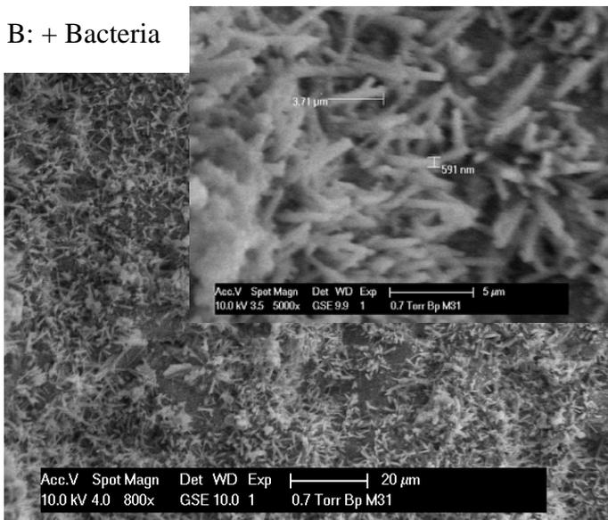
Figure 2. Concrete samples incubated in yeast extract- and peptone-containing medium. A: Control (concrete with no bacteria added) and B: Concrete containing  $10^9 \text{ cm}^{-3}$  *B.pseudofirmus* endospores. The inset in Figure 2B (5000x magnification) shows a close up of the massive calcite-like crystals formed on the concrete surface.
