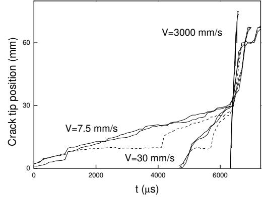
Figure 7: The crack tip position versus time for loading velocity at 7.5, 30 and 3000 mm/s respectively, where the solid lines corresponding to values measured at specimen surface, dotted lines represent values measured at specimen center.
