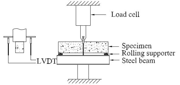
Figure 2: Experimental set-up for three-point bending tests on beams.
