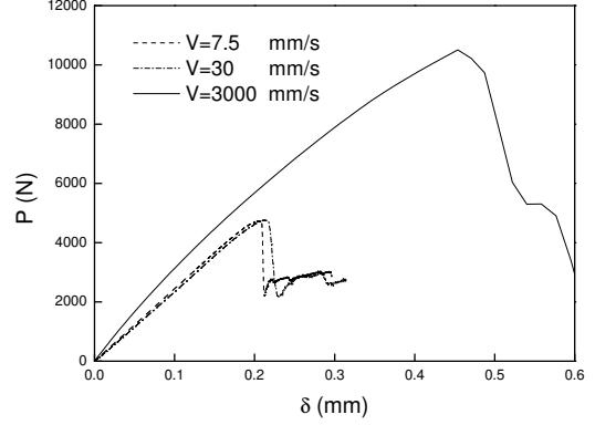
Figure 5: The load-displacement curves for loading velocity at 7.5, 30 and 3000 mm/s respectively, when static fracture properties (specific fracture energy and tensile strength) are adopted.
