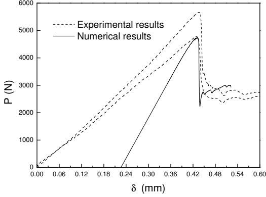
Figure 6: The numerical and experimental load-displacement comparison, when dynamic material properties (fracture energy and tensile strength) are adopted, note that the numerical curve has been translated to 0.22 mm for easier visualization of the peak load.
