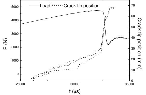
Figure 8: The zoomed view of the load history plotted against the crack tip position history for loading velocity of 7.5 mm/s.
