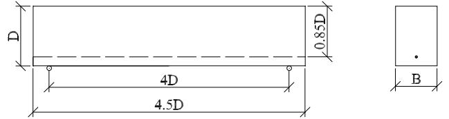
Figure 1: A reinforced concrete beam subjected to three point bending.
