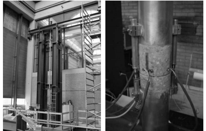
Figures 1 and 2. The Split Hopkinson Bar at the Delft University of Technology and a detail of the glued specimen and measurement system.
