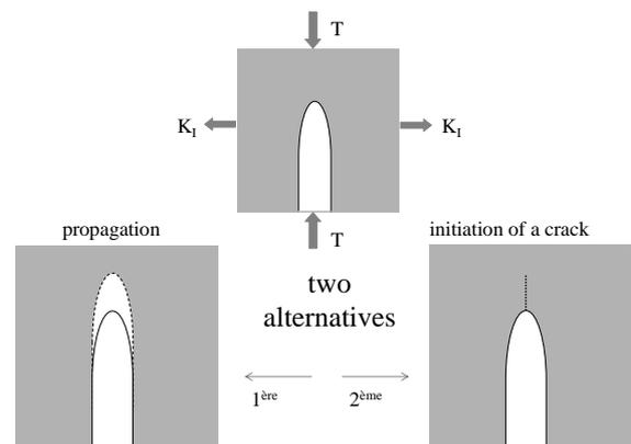
Figure 8. Stationary fracture swarm propagation or initiation of a crack at the notch tip
