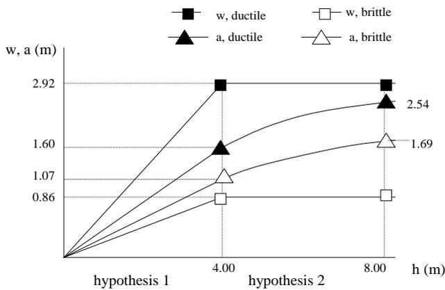
Figure 4. Results of the numerical model, spacing  $w$  and fracture length  $a$  as a function of layer thickness  $h$  for conditions of low hydrostatic pressure (predominant bending).
