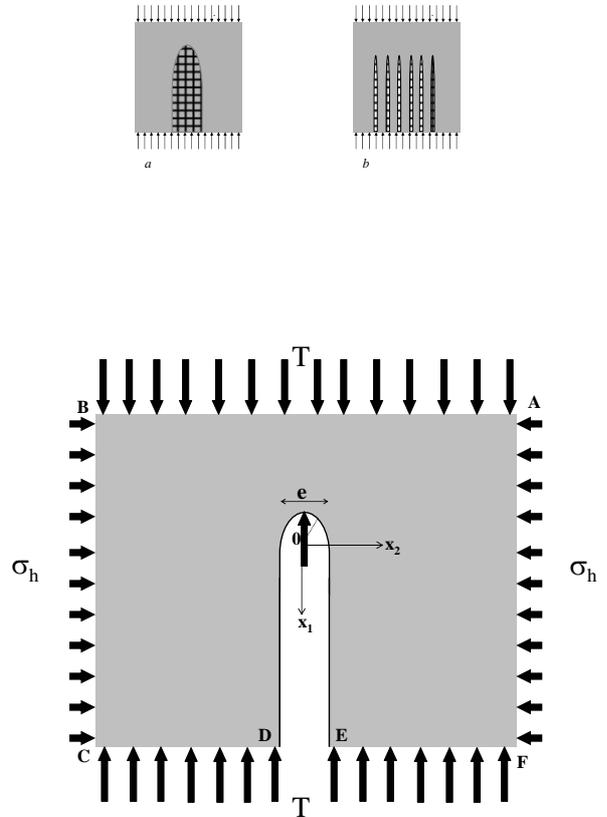
Figure 7. Figurative view of a fracture swarm (cluster)
