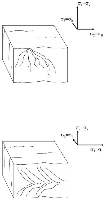
Figure 5. Schematic representation of plumose structure for vertical and horizontal propagation : non tectonic and tectonic case
