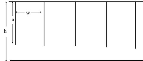
Figure 3. Fracture spacing  $w$  and length (height)  $a$  in a bed of thickness  $h$
