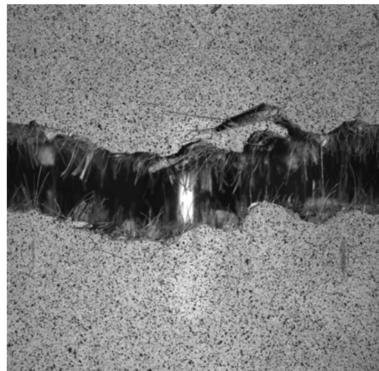
Figure 8. Final macroscopic separating crack in SHCC after failure.
