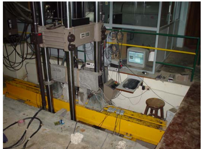
Figure 1a. Experimental set up of the three-point bend test with attached sensors.
