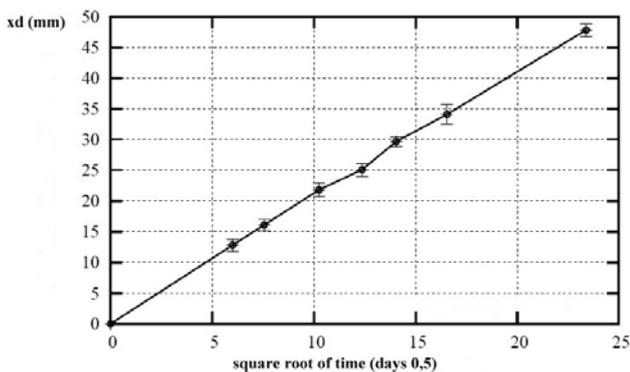
Figure 1. Evolution of degraded depth over time :  $x_d = k t^{0.5}$  where  $x_d$  is the degraded depth expressed in mm and  $t$  is time in days. This relation was established through testing without mechanical load (Nguyen, 2005).
