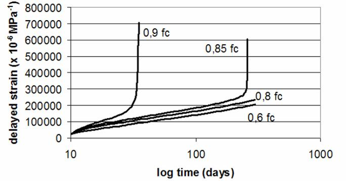
Figure 5 : evolution of the delayed strains divided by the applied stress when this stress is varying from 0.2 fc to 0.9 fc. The parameters of the Dirichlet series are those of figure 4. For the damage model  $A_c=1.5$ ,  $B_c=1500$ ,  $K_0=120 \cdot 10^{-6}$  (Mazars, 84).
