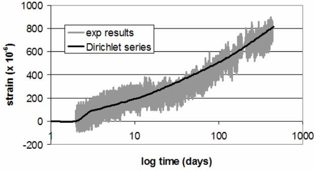
Figure 4 : adjustment of the Dirichlet series to the basic creep of concrete -  $n=7$ ;  $t_1=0,002$  d;  $t_2=0,02$  d;  $t_3=0,2$  d;  $t_4=2$  d;  $t_5=20$  d;  $t_6=200$  d;  $t_7=2000$  d;  $J_0=1/36.2$  GPa $^{-1}$ ;  $J_1=1/800$  GPa $^{-1}$ ;  $J_2=1/800$  GPa $^{-1}$ ;  $J_3=1/400$  GPa $^{-1}$ ;  $J_4=1/200$  GPa $^{-1}$ ;  $J_5=1/50$  GPa $^{-1}$ ;  $J_6=1/25$  GPa $^{-1}$ ;  $J_7=1/17$  GPa $^{-1}$ .
