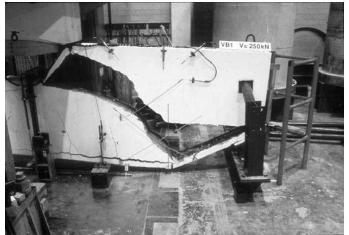
Figure 2: Shear failure of a deep beam tested at the University of Toronto.
