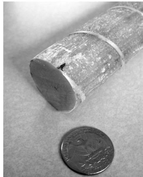
Figure 1. Ø32 mm GFRP reinforcing bar.
