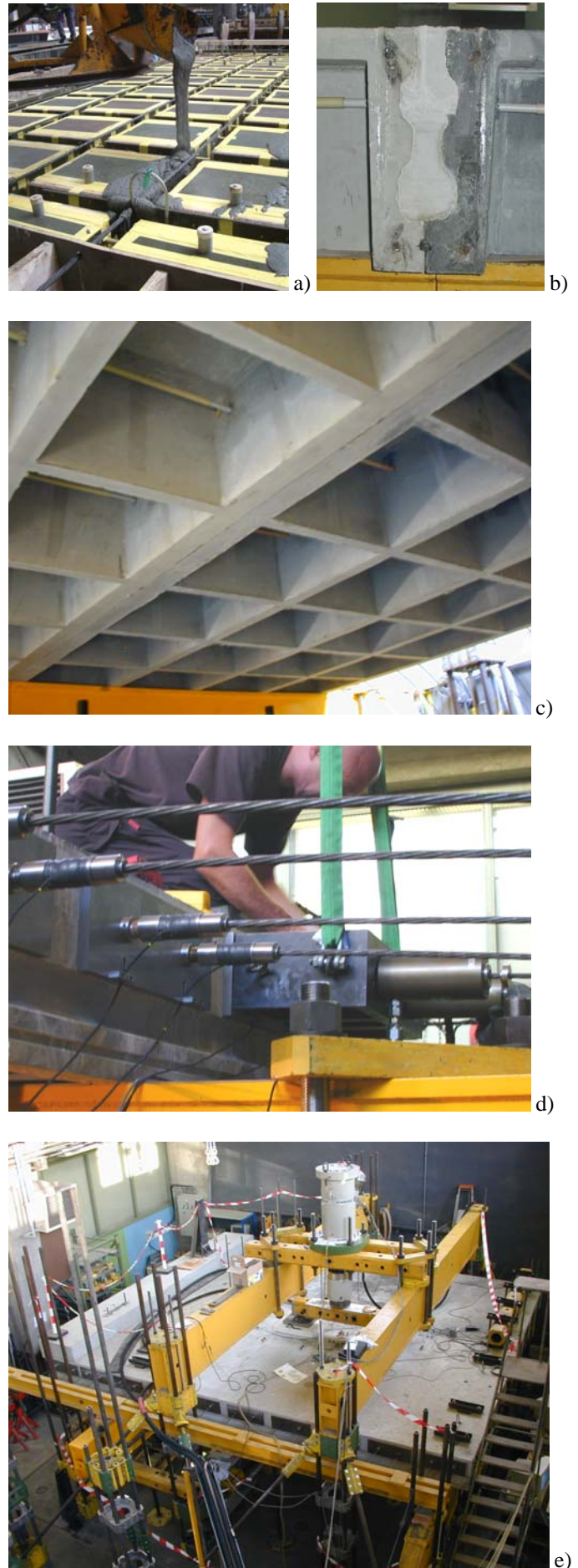
Figure 3. Model ribbed slab for validation tests. a) Casting – b) Cold joint – c) Honeycombs ; in the center, the connected side ribs of the segments – d) Longitudinal post-tensioning – e) Overview of the model under general ‘axle’ bending test.
