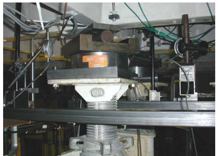
Figure 6. Support detail and reaction load measurement.
