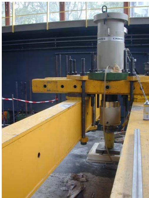
Figure 8. Fixation of the actuator and superstructures.
