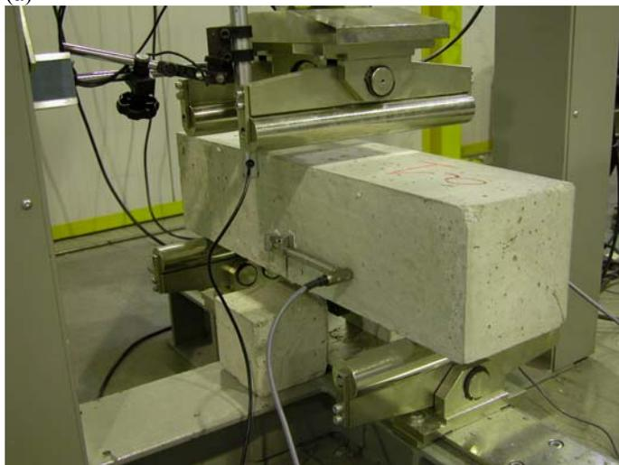
Figure 4. UNI test: (a) geometry and test set-up; (b) specimen image during testing.
