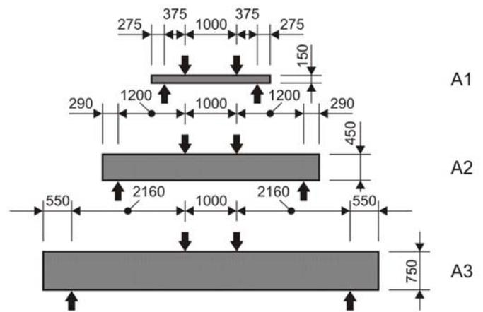
Figure 4. Size effect tests on slender beams, series A (Walraven, 1978).
