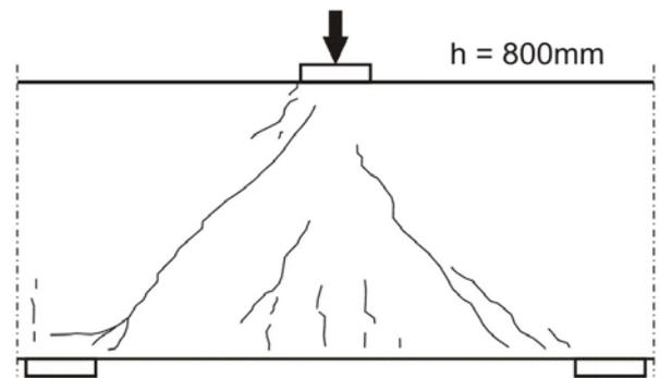
Figure 11. Failure of compression strut at the junction with the loading area.
