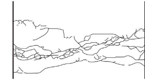
Figure 2. Crack band in a concrete with  $d_{\max} = 16\text{mm}$  (van Mier, 1996).
