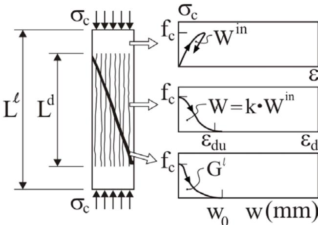
Figure 3. CDZ-model according to Markeset (1993) illustrated for a specimen loaded in concentric compression.
