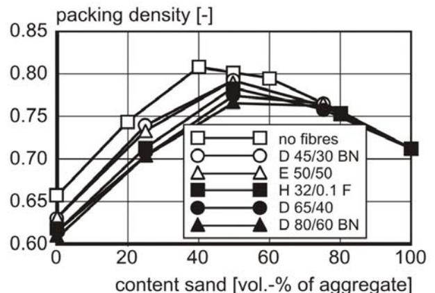
Figure 17. Effect of the sand content and the type of steel fibres (at 1.5 Vol.%) on the packing density (fibre types: first index:  $L_f/d_f$ ; second index:  $L_f$ ), according to Grünewald, 2004.
