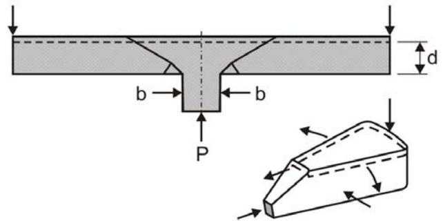
Figure 13. Mechanical model by Kinnunen and Nylander (1960) describing punching shear.
