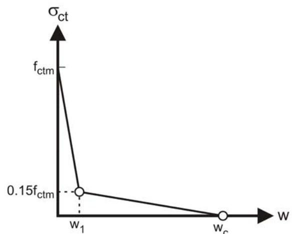
Figure 1. Stress-crack opening relation according to CEB-FIP Model Code 1990
