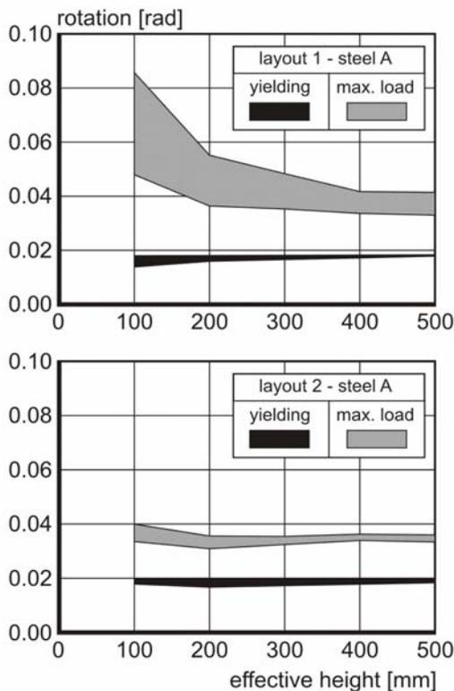
Figure 16. Calculated rotation at the onset of yielding of the reinforcement and at maximum load as a function of the effective member depth and the reinforcement layout, for a longitudinal reinforcement ratio of 0,25%, after Bigaj (1999).
