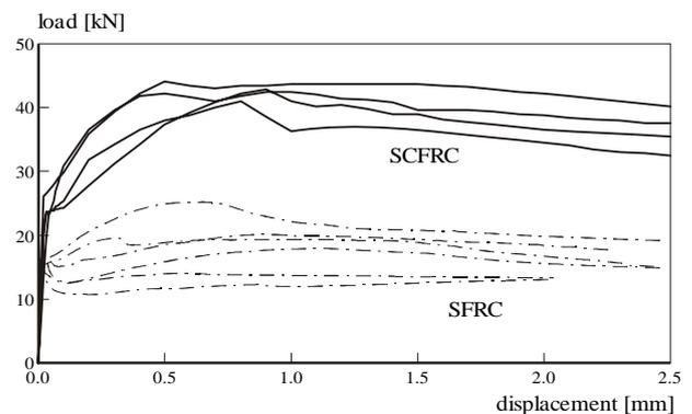
Figure 20. Test results of three point bending tests on self compacting concrete and conventional concrete, with the same concrete strength and the same amount of fibers, according to Grünewald, 2004.
