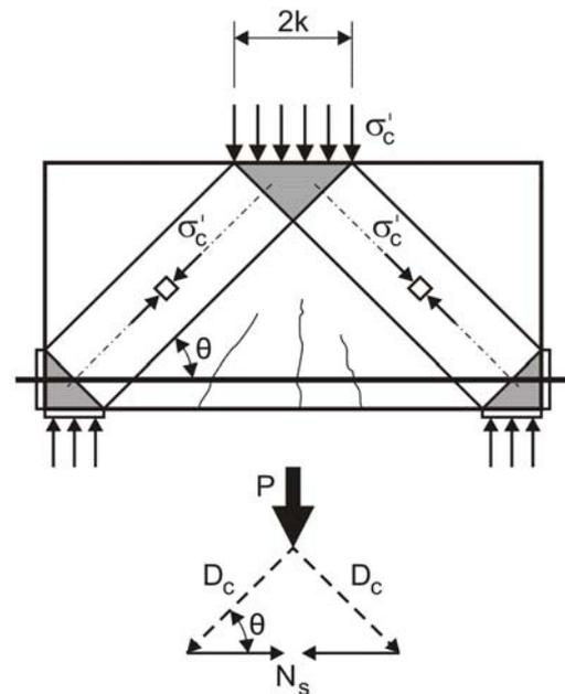
Figure 8. Strut and tie model for short deep beam loaded by a concentrated load at midspan.
