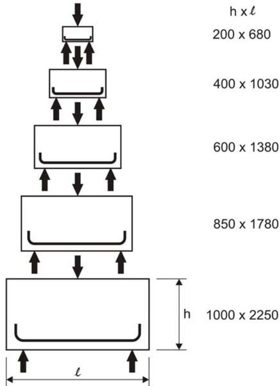
Figure 9. Shear tests on small beams with the same geometry but different size, Lehwalter, 1988.
