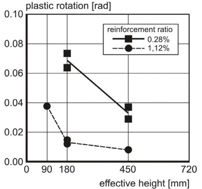
Figure 15. Observed plastic rotations at peak load versus effective depth of the beams (Bigaj, 1999).
