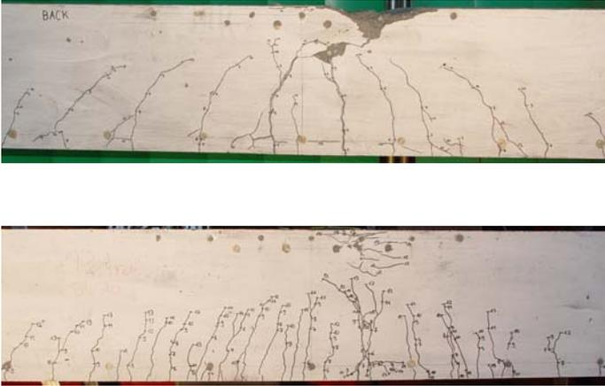
Figure 23. Plastic hinge in plain concrete (top) and fiber reinforced concrete (bottom) (Schumacher, 2006).
