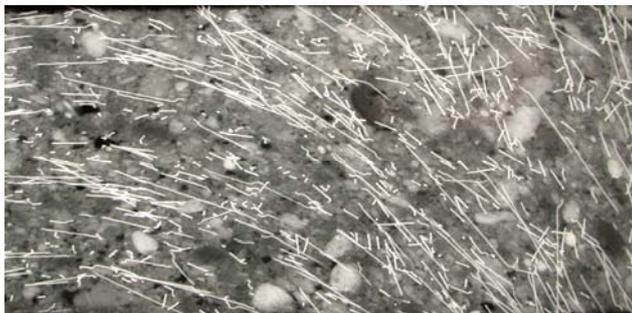
Figure 21. X-Ray photo of fiber orientation in tunnel element, cast with self compacting fiber concrete
