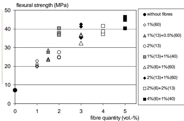
Figure 18. Flexural tensile strengths of various types of hybrid fiber concrete, Markovic, 2006.
