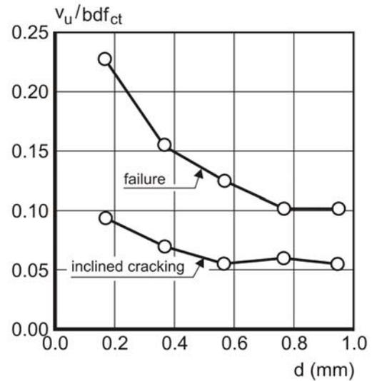
Figure 10. Relative shear stress at inclined cracking and at failure for short deep beams with  $a/d = 1$ .
